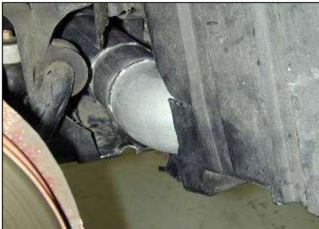
l. Trim inner fender liner and under tray as shown for proper fit.
