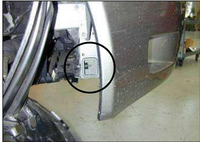
g. Install the supplied rubber mount into the passenger side radiator support frame rail as shown. When tightening the nut, tighten until the thin outer wall of the support starts to deflect (See step 3h for a closer view).
