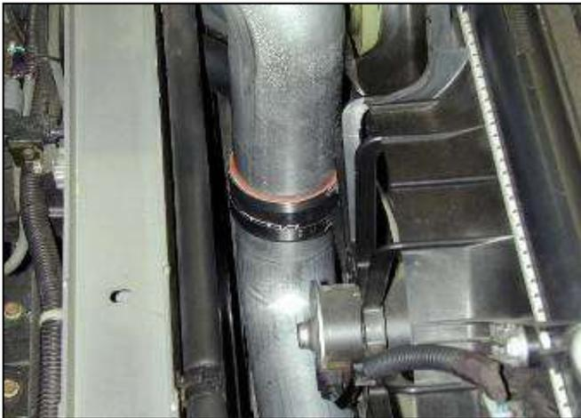
j. Using the 3.25" silicone hose and two #48 hose clamps supplied, attach the upper and lower intake pipes together.
