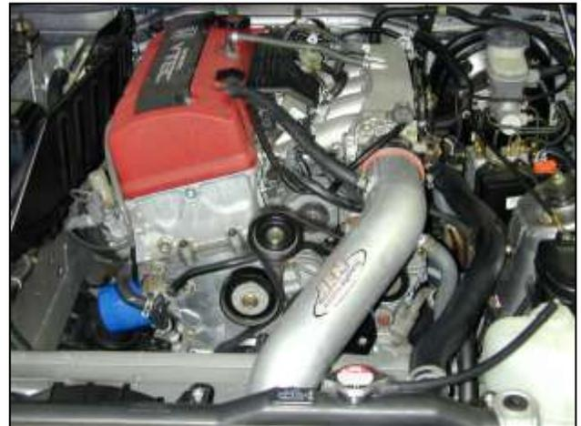
o. Ensure the air filter is not touching any part of the vehicle. Position the inlet pipe for best fitment. Be sure that the intake pipe or any other component is not in contact with any part of the vehicle. Tighten the hose clamps at the throttle body and silicone coupling. Tighten the nut on the mounting bracket. Check for proper hood clearance. Re-adjust pipe if necessary.
