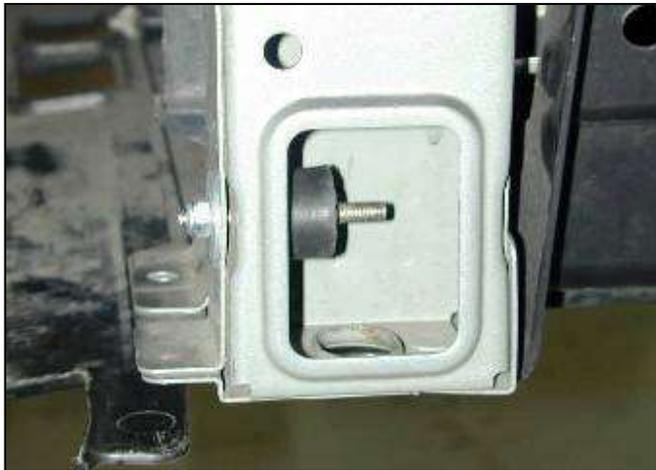
h. Install the supplied rubber mount into the passenger side radiator support frame rail as shown. When tightening the nut, tighten until the thin outer wall of the support starts to deflect.
