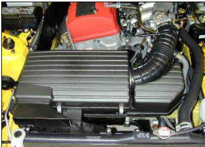
Factory air box system installed
