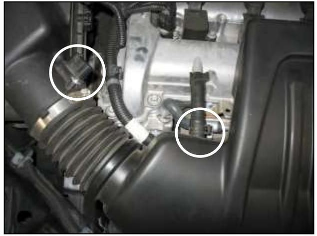
f. Release the mass air flow sensor wire from the mass air flow sensor located in the inlet tube. Also release the air breather hose clamp from the stock inlet tube.
