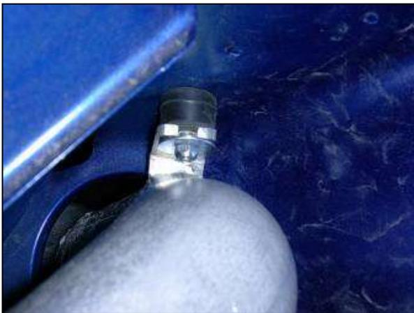
e. Use the supplied washer and serrated nut to secure the intake pipe. Install the air filter on the end of the pipe within the fender well. Secure the air filter to the intake pipe.
