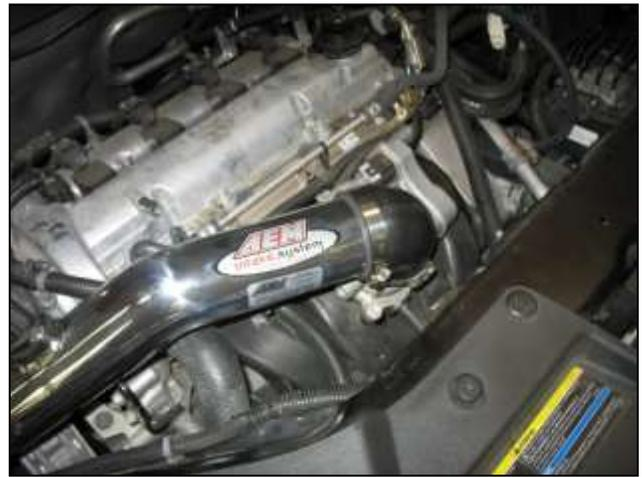
d. Assemble the intake pipe with the supplied 90 degree coupler and two #44 hose clamps. Line up the intake pipe bracket with the rubber mount. Then slide the coupler over onto the throttle body. Do not completely tighten the hose clamps or mounting hardware yet.
