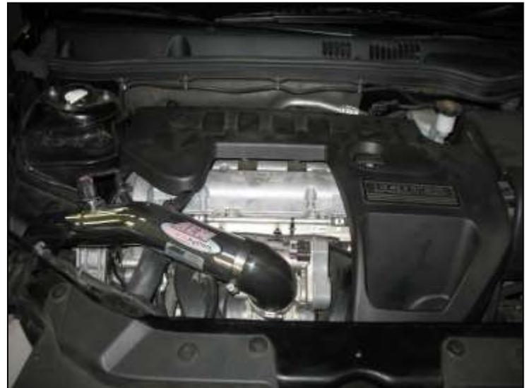
AEM® intake system installed
