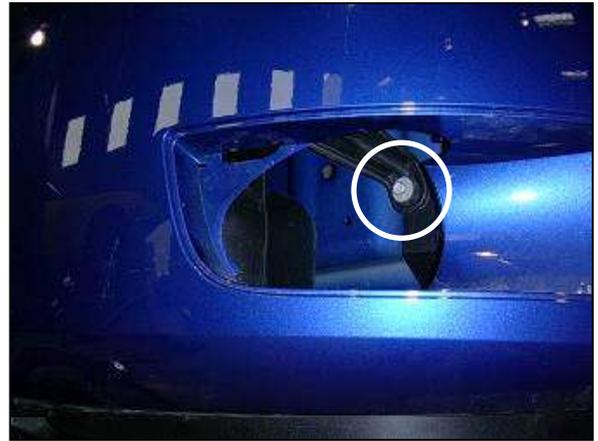
j. Remove the bolt at the front of the lower air box. Remove the lower air box from the vehicle. On the 2006 Cobalt you will need to gain access to this bolt by removing the front part of the fender liner and going underneath the car. After removing this bolt remove the lower box from the vehicle.
