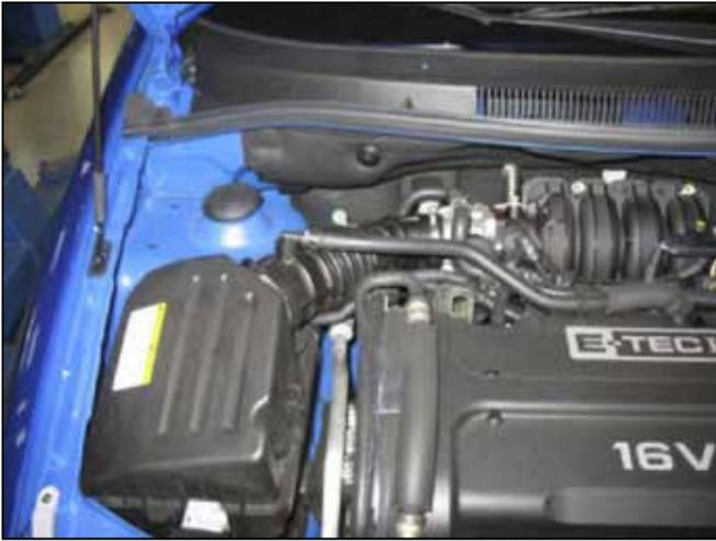
Stock air box system installed.
