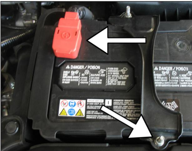
f. Remove the battery by removing the battery tie down and disconnecting the positive terminal.
