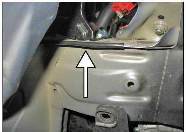
f. Apply the rubber edge trim onto the frame rail as indicated.
