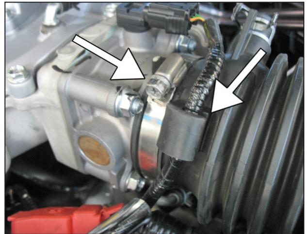
g. Loosen the hose clamp securing the inlet tube to the throttle body. Also, remove the wiring harness from the inlet tube.
