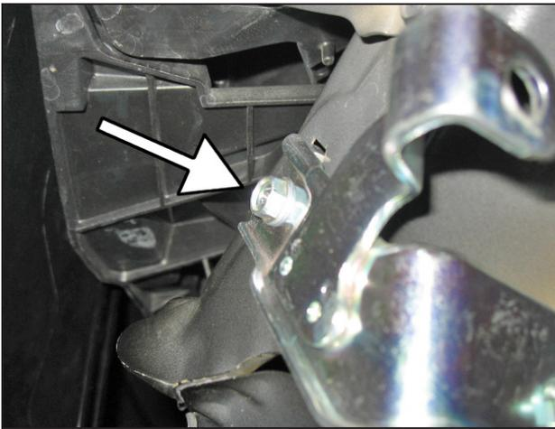
w. Locate and remove the 10mm bolt holding the remainder of the air box system to the chassis.
