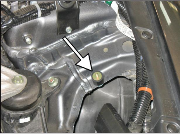
g. Insert one of the 1" rubber mounts (1228599) into the indicated area. Secure with a supplied 6mm fender washer and serrated nuts.
