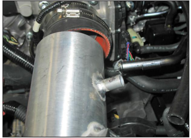
h. Insert the upper intake pipe (2-6831) into the previously installed reducer coupler on the throttle body. The end of the intake pipe closest to the PCV nipple and MAF adapter should install into the throttle body coupler. Secure in place with a hose clamp (9452).
