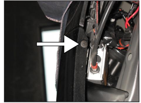
v. Remove the front bumper by removing the side and bottom clips as indicated. Please do not forget to remove the Phillips screw (picture on the far right) from both the left and right side of the vehicle. If the vehicle is equipped with fog lights, unplug them before removing the bumper.
