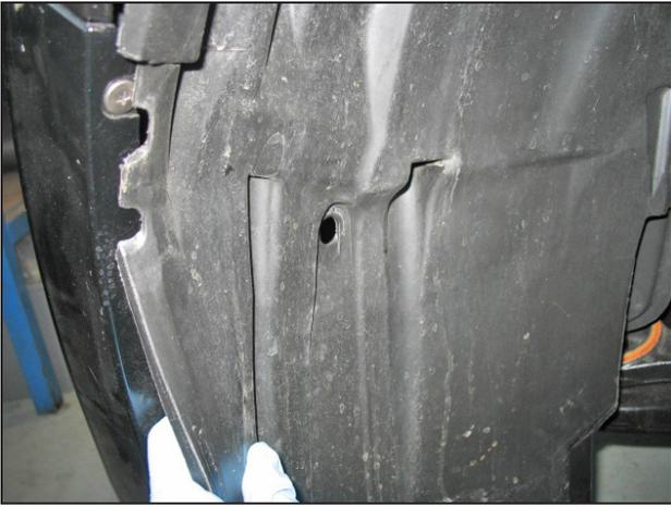
t. Wheel well liner and bottom plastic tray: Install the wheel well liner, bottom plastic tray and any hardware that was removed during steps 2p-2q. **NOTE: Failure to install the fender liner will result in diminished performance and increase the potential for engine damage due to water ingestion in rainy conditions.**
