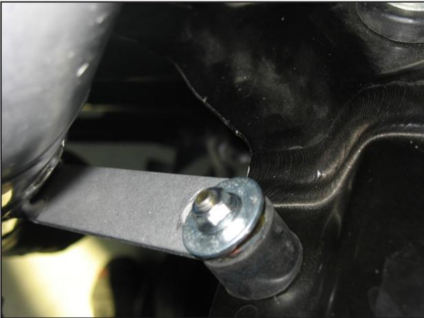
i. Slide the upper intake pipe's bracket onto the previously installed rubber mount; loosely secure with a 6mm washer and nut.
