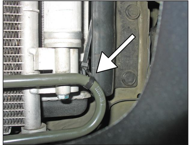
l. Insert the tab of the zip-tie (1-127) into the hole on the radiator support. Wrap the zip-tie around the condenser coil and tighten so the coil is pulled inward approximately 10mm.
