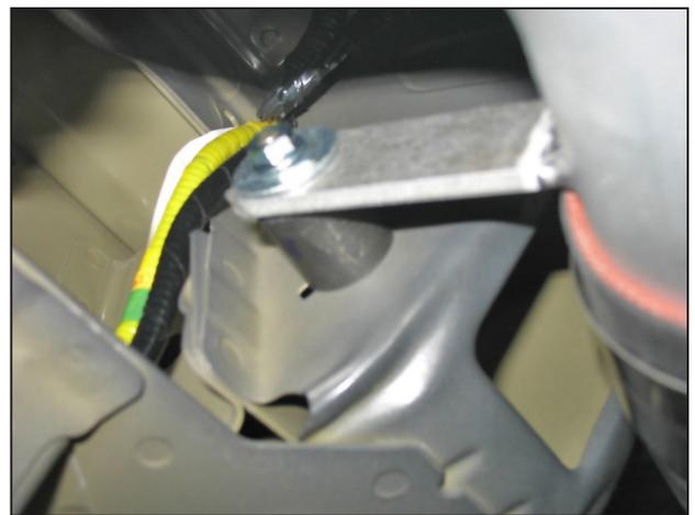
p. Slide the lower intake pipe's bracket onto the rubber mount that was installed in step 3m. Secure the rubber mount with the provided 6mm fender washer and nut.
