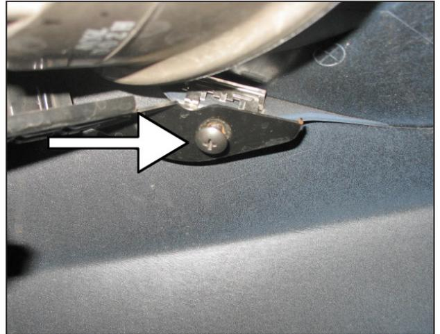
b. Locate the driver side fog light bracket, it is clipped onto the front bumper. Remove the three mounting screws shown in the photos.
