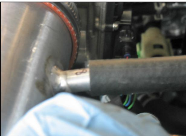
k. Connect the other end of the 1/2" hose to the upper intake pipe's nipple and secure with the provided hose clamp (08407).
