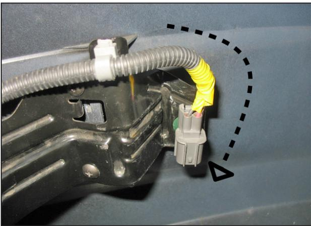
c. With the foglight removed from the bumper, bend the fog light bracket in the orientation shown in the diagram.
