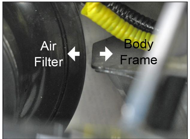
q. From previous steps 3i and 3p, adjust the brackets to allow clearance in the indicated areas shown in the photos.
