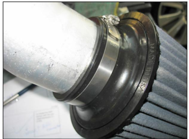
n. Install the air filter element onto the non-bracket side of the lower intake pipe (2-6832). Secure in place with the provided hose clamp (9456).
