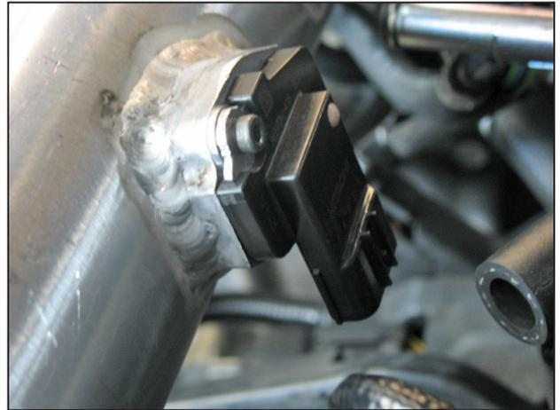
j. Install the MAF sensor with the factory hardware; connect the wire harness to the MAF sensor.
