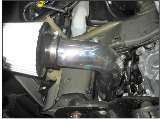
o. Install the air filter onto the lower end of the lower intake pipe. Once proper fitment is achieved secure the air filter to the intake pipe with a #9452 hose clamp.
