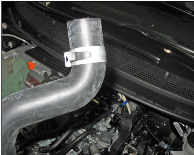
e. Install the supplied radiator hose using the stock hose clamps.
