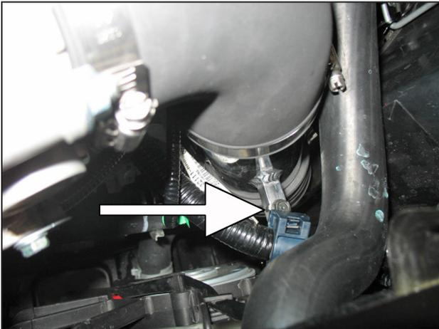
j. Install bracket #32-3058 onto the upper intake pipe's bracket with the supplied bolt #1-2110. Attach the blue harness to the metal clip.
