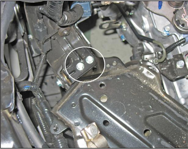
n. Remove the lower inlet tube and the bracket securing the positive battery cable. The bracket securing the positive battery cable has two bolts that will need to be removed.
