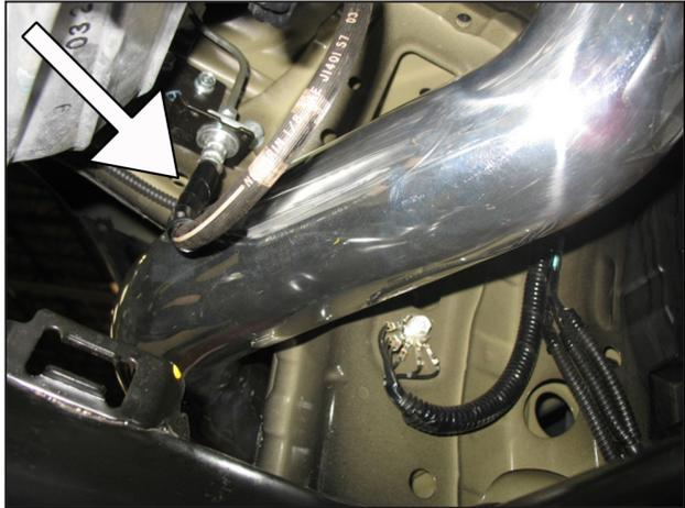
m. Install the supplied helical wrap onto the clutch line where the lower intake pipe passes.
