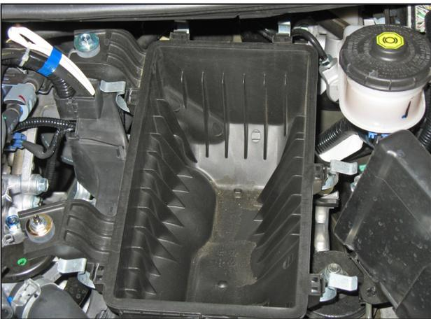
g. Remove the upper air box and air filter from the lower air box. Remove the two bolts and one nut securing the lower air box to the vehicle.
