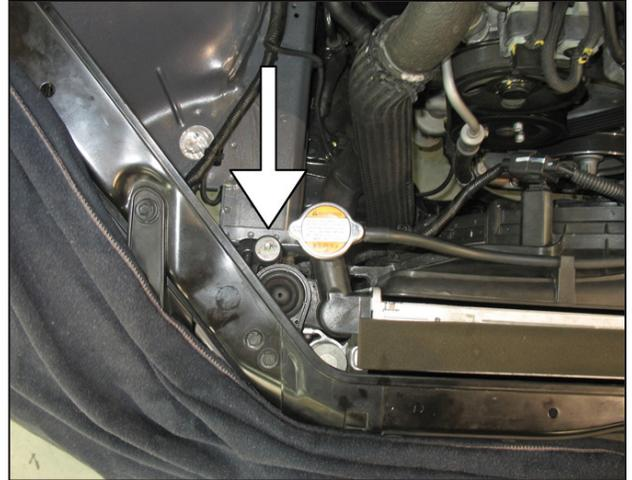
c. Install the M6 rubber mount in the location shown.
