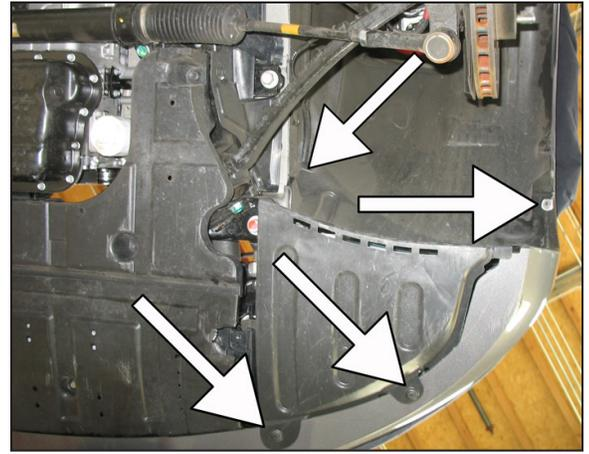
u. Reinstall the inner wheel liner with the three clips and one screw removed in step 2f.
