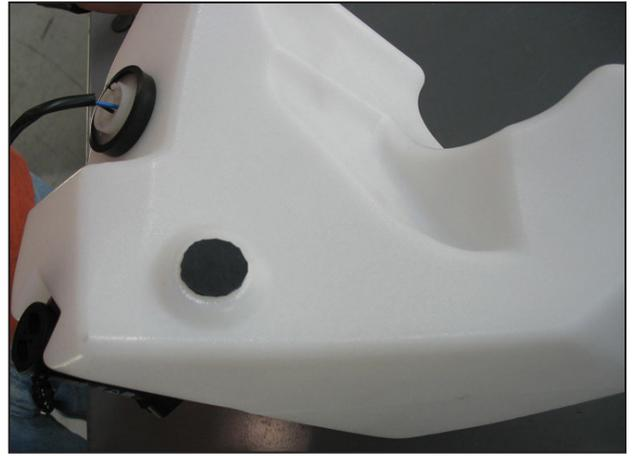
q. Stick the self-adhesive rubber pad onto the small bump that protrudes from the washer bottle.
