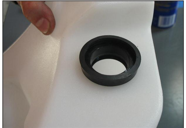
o. Install the level sensor grommet into the supplied washer bottle as shown.
