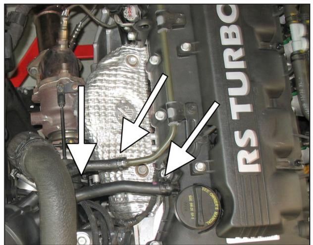
d. Loosen the hose clamp at the compressor inlet. Locate the two breather hoses connected to the valve cover inlet nipples, compress the spring clamps and slide them off the inlet nipples so the hoses can be removed.
