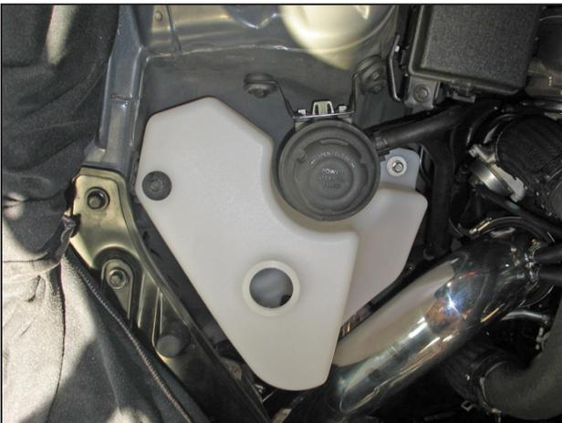
r. Lower the washer bottle assembly into place as shown. Plug the washer hose and wire harness connector to the pump. Plug in the level sensor connector and tuck the wires away. Secure the washer bottle into place with the two M6 bolts removed in step 2h.
