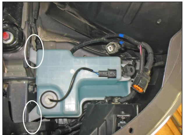
h. Remove the two M6 bolts securing the washer bottle. Unplug the hose from the washer pump and remove the washer bottle from the vehicle. Drain the washer fluid into a clean container and set the washer bottle aside.
