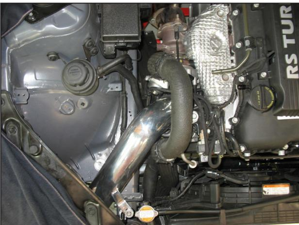
d. Install the inlet pipe by lowering the front end into position, then insert the rear end into the compressor inlet coupler. Guide the pipe's bracket into position on the rubber mount and secure with a M6 nut and washer. Leave the M6 nut loose for now.
