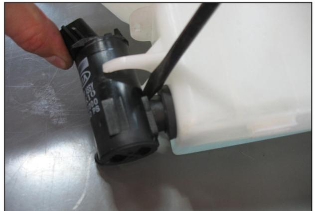
k. Pry the washer pump out of the grommet and set it aside. Also remove the grommet and set it aside.
