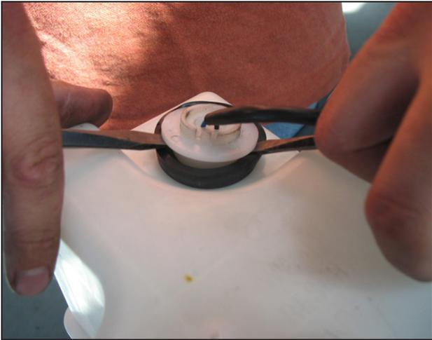
l. Using two flat head screwdrivers, carefully pry up on the lip of the washer level sensor, using care not to damage the rubber grommet. A soapy water mixture may be used to aid with the sensor removal. Also, remove the grommet and set aside in a safe area.
