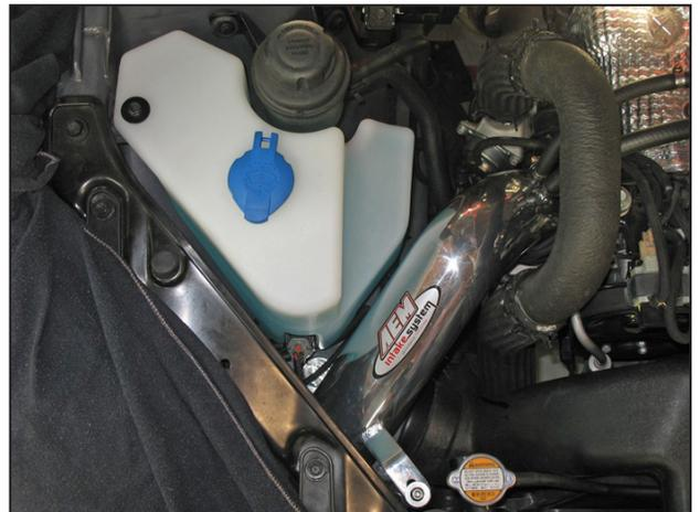
s. Refill the washer bottle with the washer fluid drained in step 2h. Snap the blue cap onto the neck of the washer bottle.
