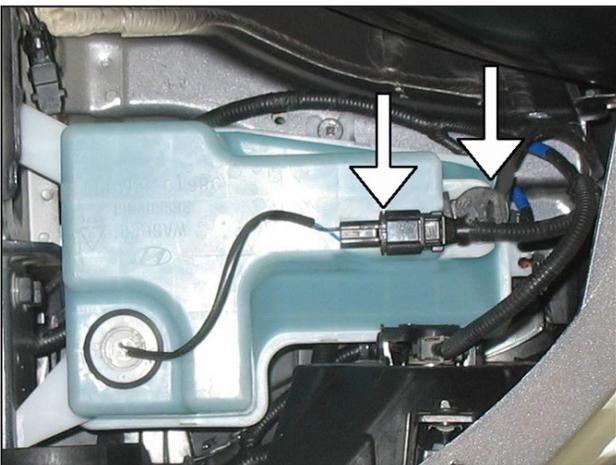
g. Unplug the washer pump and washer fluid level sensor.
