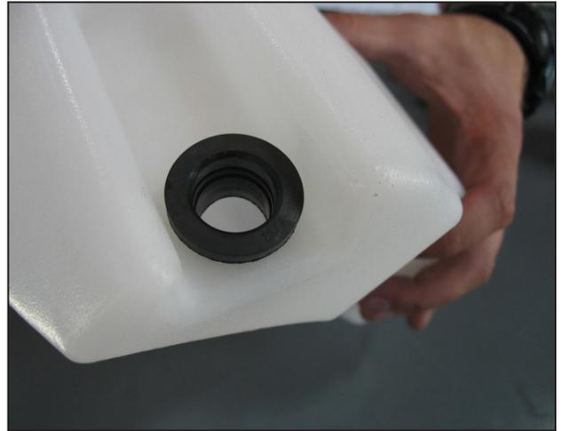
m. Insert the stock washer pump grommet into the inlet on the front of the supplied washer bottle.
