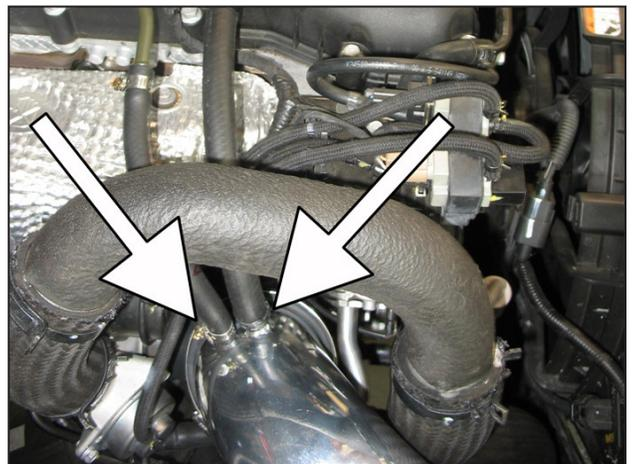
e. Install the larger diameter breather hose to the inlet pipe and valve cover nipple. Secure the large breather hose using the stock spring clamps. Install the smaller diameter breather hose to the inlet pipe and hard line using the two small hose clamps supplied with the kit.
