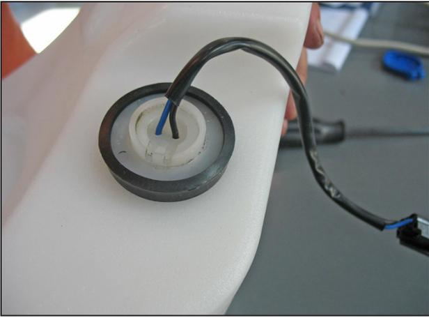
p. Apply a liquid soap solution to the level sensor and insert it into the grommet. Make sure that the level sensor is pressed all the way into the grommet. The lip of the sensor should sit inside the groove of the grommet.
