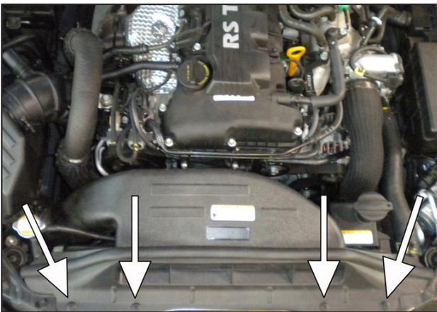
a. Remove the four clips securing the air scoop, remove the air scoop from the vehicle.
