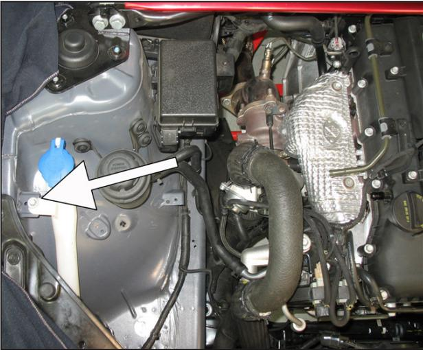
e. Remove the M6 bolt securing the washer bottle filler neck. Also unplug the passenger side headlight.
