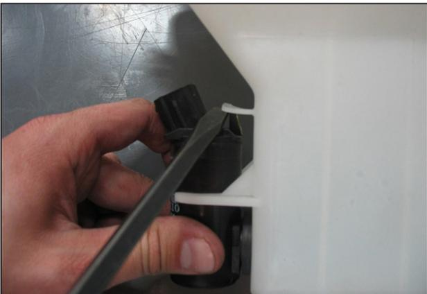
j. Using a flat head screwdriver, unclip the washer pump from the washer bottle as shown.
