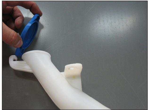
i. Remove the blue washer fluid cap from the stock washer bottle neck.
