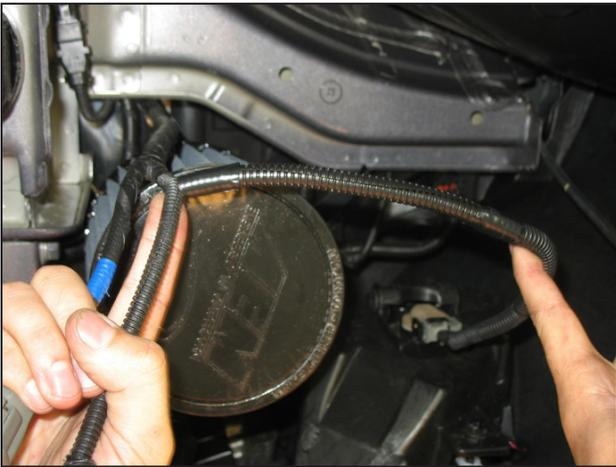
h. Wrap the supplied convoluted slit over the exposed fog light wires and secure with electrical tape. Unclip the washer fluid hose from the clip that attaches it to the inner fender. Push the hose and the two wire connectors up top behind the headlight.
