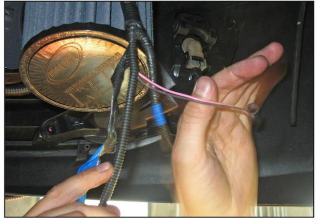
g. If the vehicle is equipped with fog lights, un-wrap the convoluted slit to expose the wires, then remove the fog light wires.
