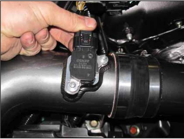
n. Plug in the MAF sensor wire connector into the MAF sensor.
