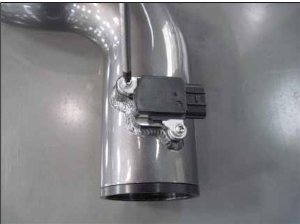
d. Install the MAF sensor using the stock screws.
