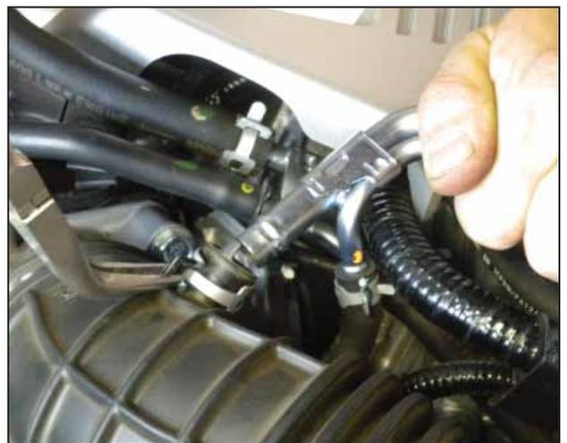
j. Release the spring clamp and remove the PCV hose from the inlet tube.
