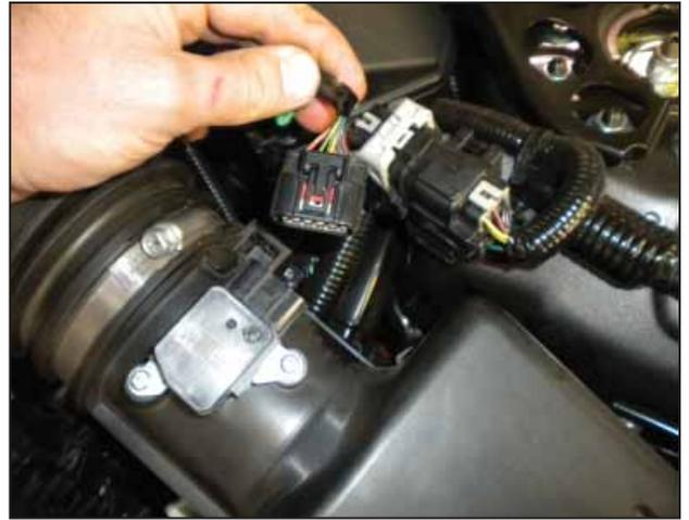
f. Disconnect the MAF sensor wire connector from the MAF sensor.
