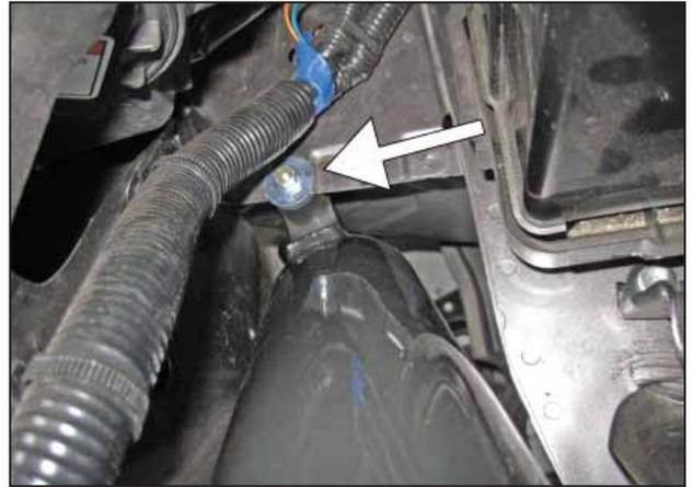
k. Secure the rubber mount previously installed on the intake tube bracket with the provided M6 washer and nut as shown.
