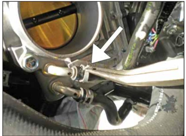
z. **CAUTION: Ensure the engine is completely cool before removing the coolant hose, or hot coolant will escape from the cooling system and cause injury or damage. Be sure to capture any lost coolant in a clean container.** Release the spring clamp on the throttle body coolant line.
