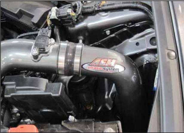
j. Install the lower intake tube as shown.
