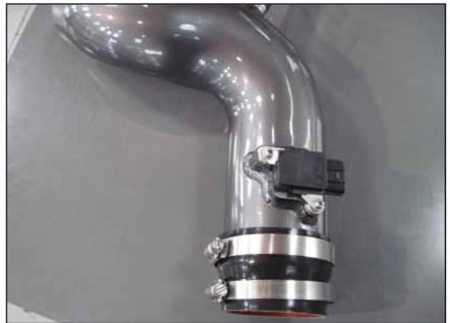
g. Install the reducer coupler on the MAF side of the intake tube.
