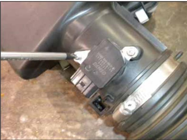
y. Remove the two Phillips screws and remove the mass air sensor from the air box assembly.
