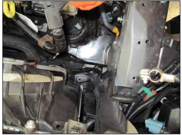
x. Remove the battery tray and intake duct.
