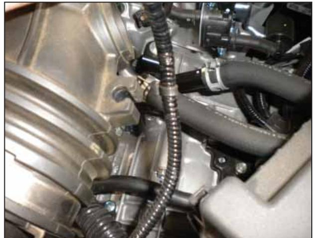
h. Remove the MAF sensor wire from the inlet tube.
