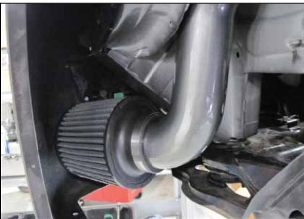
l. Install the AEM® Dryflow™ air filter.
