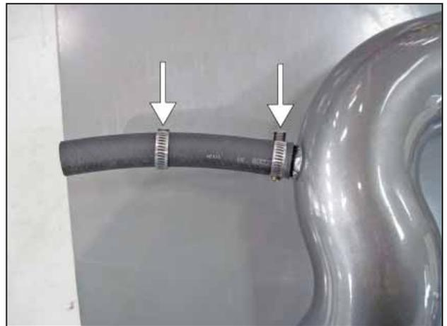
e. Install the supplied 5/8" PCV hose and secure to the intake pipe with the hose clamps as shown.
