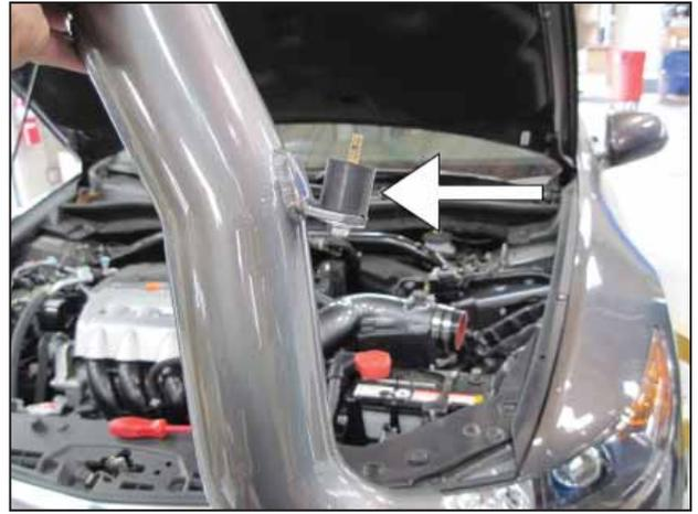
i. Attach the supplied rubber mount onto the lower intake tube bracket as shown.
