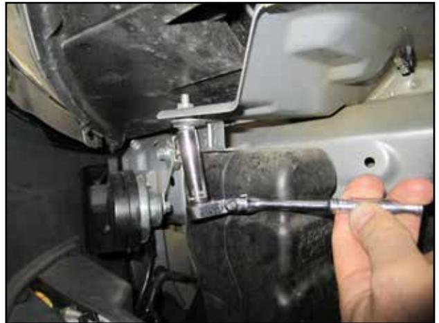
n. Remove the top 6MM bolt holding the lower resonator in place.
