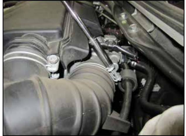
b. Loosen the hose clamp on the throttle body.
