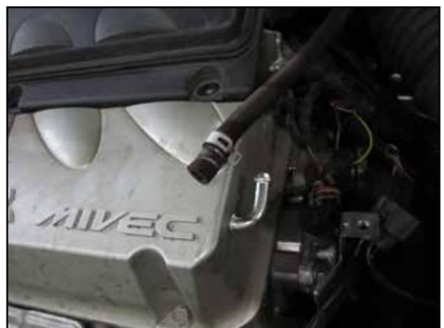
d. Release the clamp on the valve cover for the PCV hose, then remove the hose from the valve cover.
