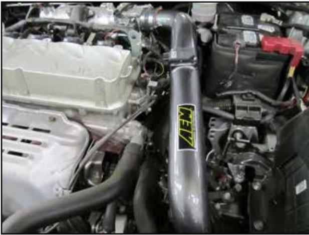
e. Now install the AEM intake tube (A).
