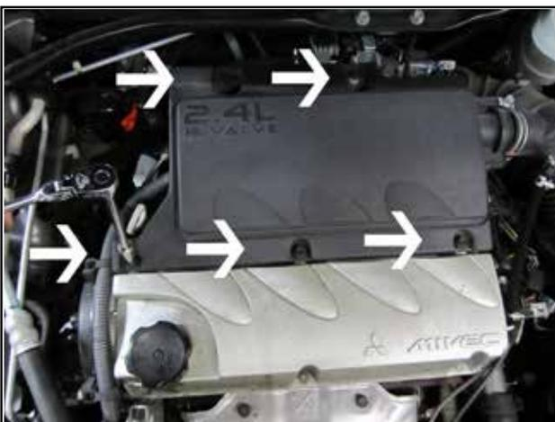
c. Loosen and remove the five 6MM bolts holding the resonator on the valve cover.
