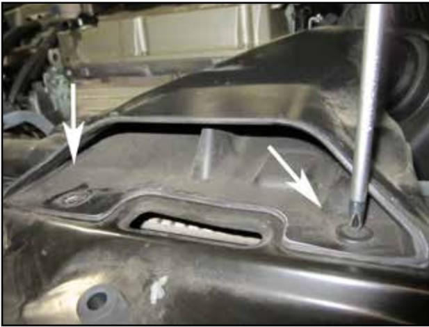
e. Remove the two plastic fasteners holding the stock air scoop. Remove the air scoop.
