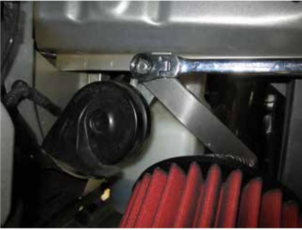
k. Tighten the 8MM nut on the intake bracket tube as shown.
