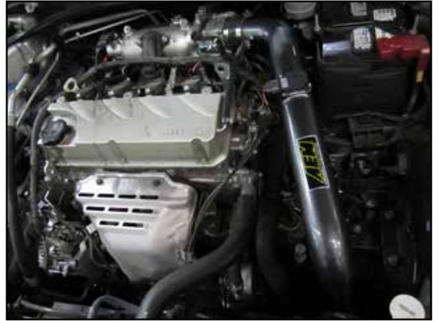
l. Check the fitment of the intake system and ensure there is clearance between the inlet pipe and its surrounding components. Once proper fitment is achieved check all the hose clamps and M8 nut on the rubber mount.
