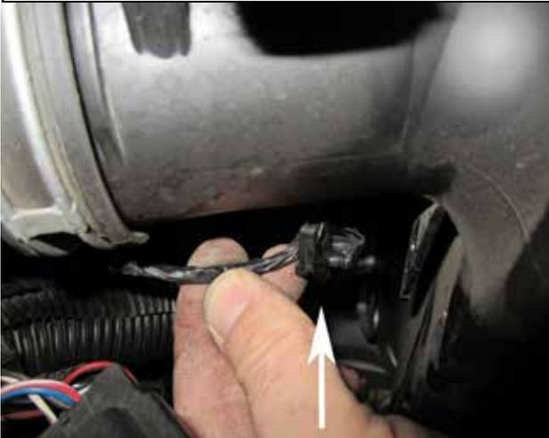
g. Release the (MAF) wire harness clip on the air box as shown.
