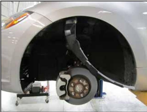
m. Move the fender liner out of the way to gain access to the fender well.
