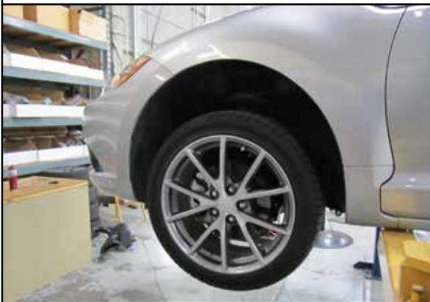
i. Raise the front of the vehicle with a jack. Support your vehicle using properly rated jack stands before wheel removal or while working under the vehicle.
