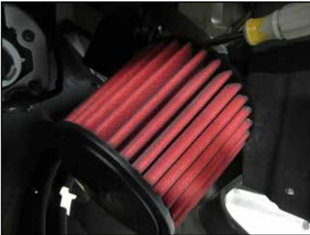
g. Install the AEM dryflow filter (I).
