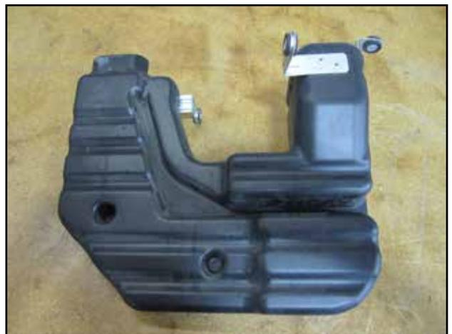
p. Remove the resonator from the vehicle, this is what the resonator looks like when removed.
