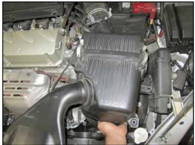
h. Lift up on the air box and remove the stock intake system.
