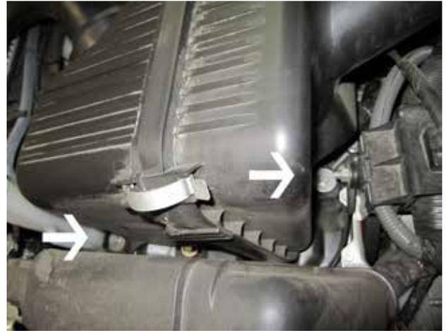
f. Loosen and remove the two 6MM bolts holding the air box in place.
