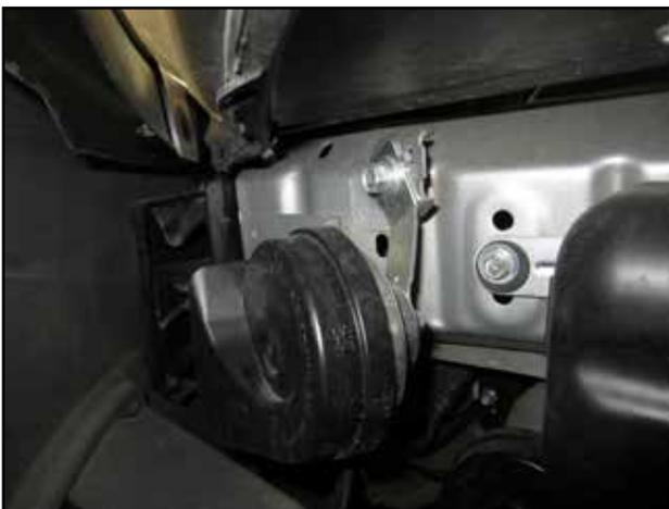
o. Remove the lower left 6MM bolt holding the resonator.
