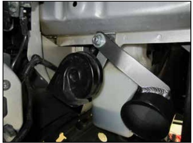
f. Use the 8MM nut (H) and washer (G) on the intake tube bracket.
