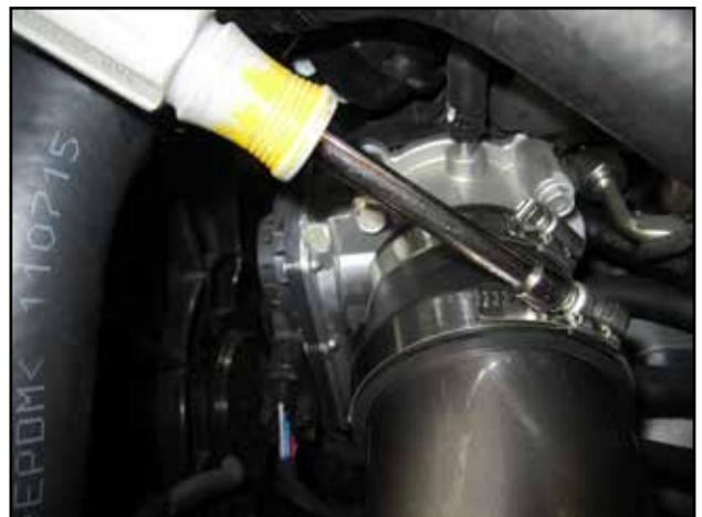
j. Make sure you have clearance around the intake tube and AEM filter and tighten the hose clamp on the intake tube.
