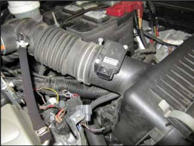
a. Unplug the (MAF) sensor. Remove the (MAF) sensor from the air filter housing.
