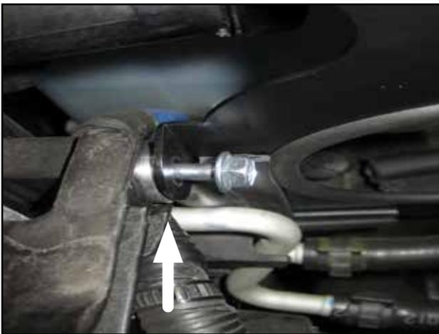
n. Install the mounting block (K) and M6 bolt (M) into the front mounting tab. Do not fully tighten at this time.
