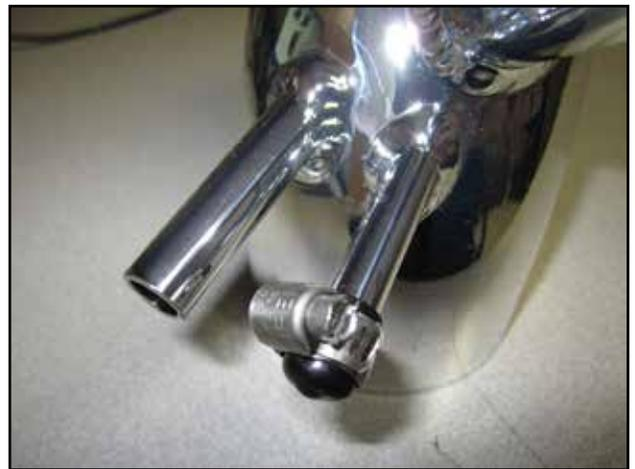
i. For automatic cars use the provided cap (R) and hose clamp (S) to cap off the vent tube.
