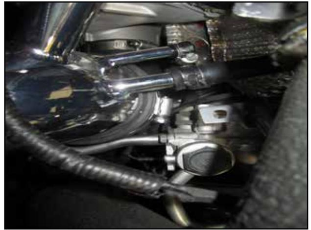
s. Reconnect the PCV hoses and fasten with the OEM spring clamps.
