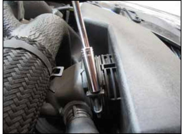
b. Loosen the hose clamp on the intake pipe.
