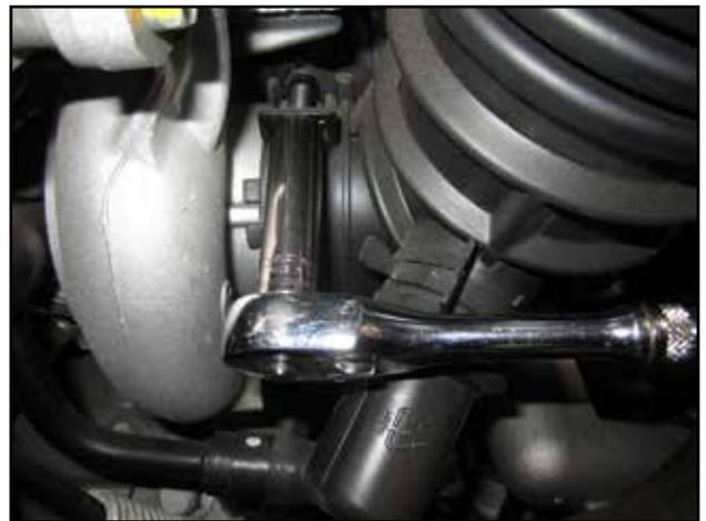
h. Loosen the hose clamp securing the stock tube onto the turbo inlet.
