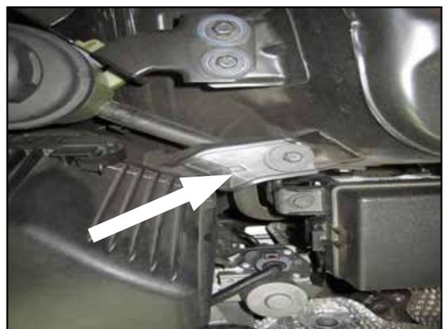
d. Remove the M6 bolt holding the airbox in place.
