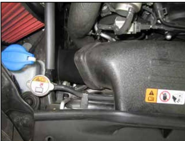
v. Install the scoop and adapter as shown.
