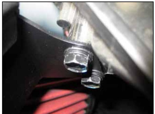
q. Reinstall the OEM M6 bolts in the factory mounting bracket location.
