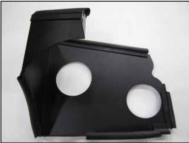
f. Install the edge trim (J) & (N) on the outer edges of the heat shield as shown.
