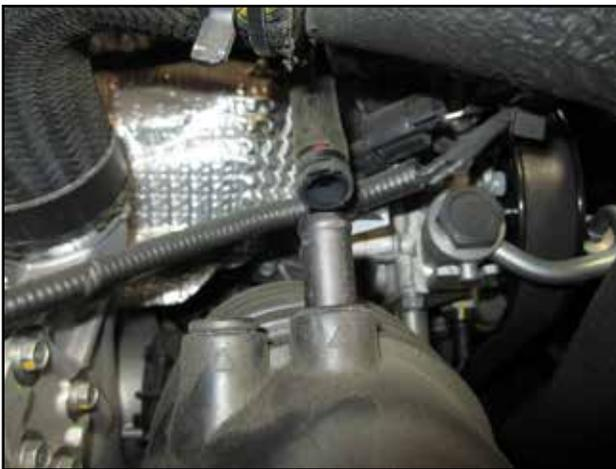
g. Release the clips on the two PCV hoses (Manual Trans) and disconnect the hoses from the intake tube. (Automatic shown)
