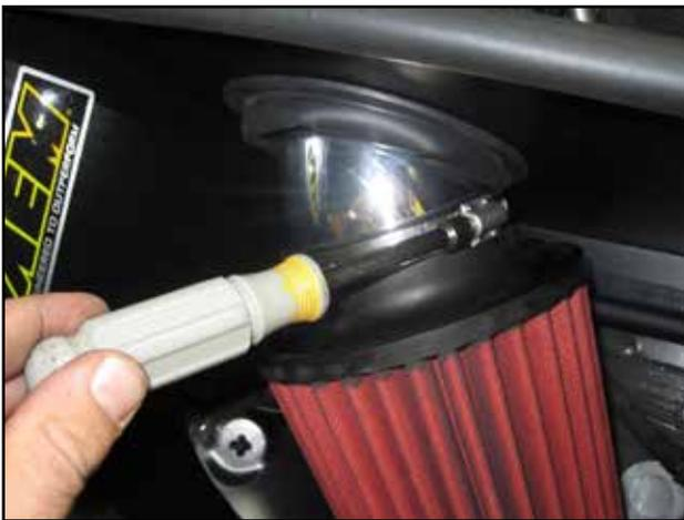
t. Align the filter and tube then tighten hose clamps (F) and (I).
