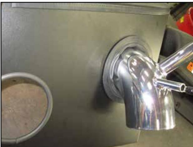
j. Place intake tube (B) through the hole in the heat shield (O) as shown.
