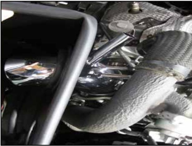
l. Install intake tube (B) into coupler (H) .
