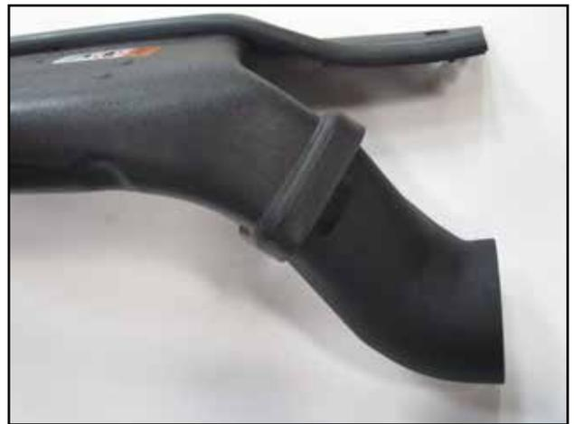
u. Install the AEM scoop adapter (A) into the OEM ducting.
