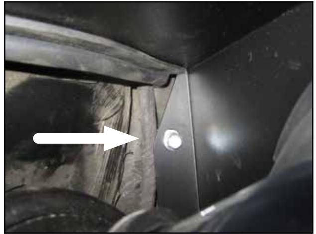
m. Install the M6 Bolt (M) and washer (Q) onto the bottom of the heat shield. Do not fully tighten at this time.
