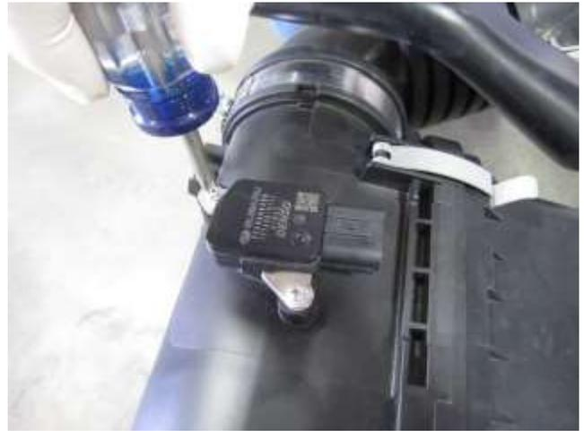
f. Remove the mass air flow sensor from the stock air box. This will be reused in 3a.
