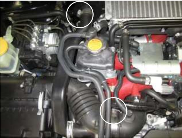
e. Loosen the hose clamps at the sound tube and the stock intake tube. Then remove the complete air box from the vehicle. **NOTE:** Do not discard your stock equipment.
