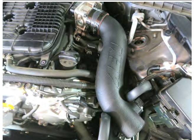
h. Install the driver side intake tube and connect the factory PCV hose. Push the tube completely into the coupler and down into the heat shield's cutout before tightening the hose clamp to 30 in-lb. Ensure clearance around tube once installed.
