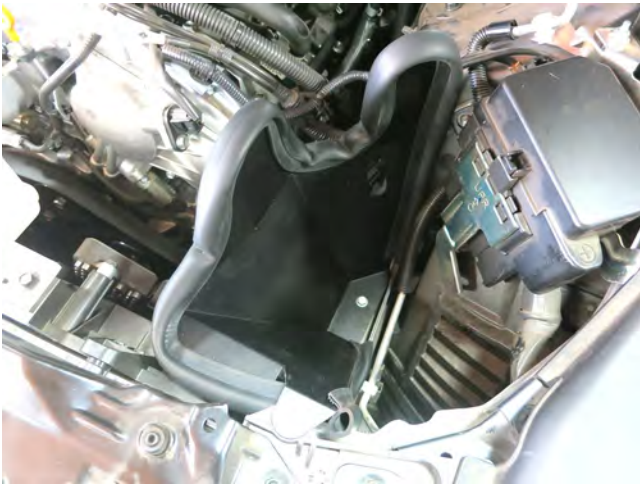
e. Install the heat shields by pushing the heatshield mount into the stock rubber grommet and bolting the front using the bolts removed in step 2d. Ensure the large wire loom is outside the heatshield when installed.
