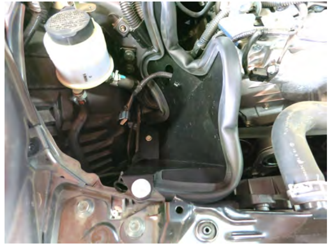
f. Pull the MAF harness through the hole in the heat shields and clip the harness to the outside of the heatshield as shown. Note: the harness clip may need to be adjusted to be secured to the heat shield.
