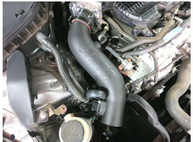
j. Install the passenger side intake tube by fully inserting the tube into the coupler and pressing the tube down into the heat shield's cutout before tightening the hose clamp to 30 in-lb.
