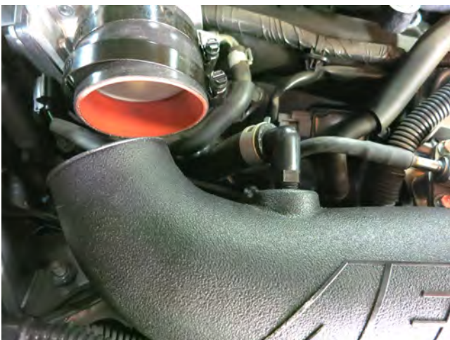
i. Lower the passenger side intake tube into the engine bay and connect the hose installed in step 3b to the intake tube and secure using the factory spring clamp.
