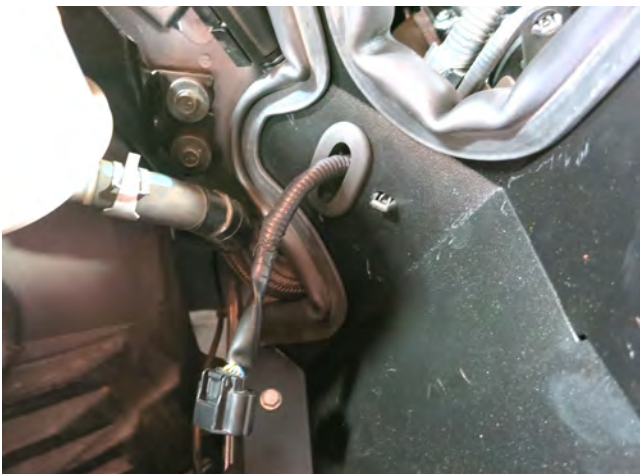
g. Slip the provided grommet over the MAF harness and fit it into the slot in the heat shields as shown.
