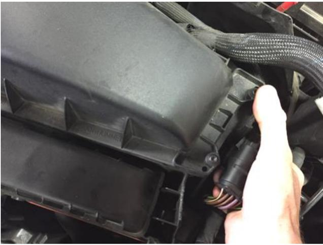
e. Lift up on wire harness retainer on the side of the airbox to remove it.
