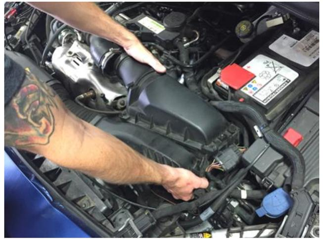
f. Lifting as shown above, remove the factory airbox assembly from the vehicle.
