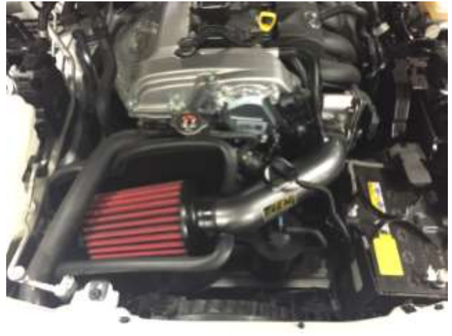
AEM INTAKE INSTALLED
