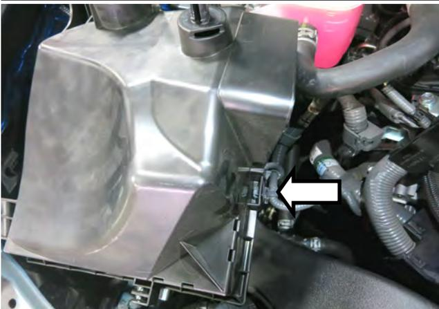
i. Flip the lower air box around. Remove the wire tie from the air box. Remove air box from vehicle.
