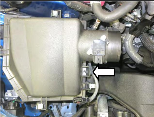
g. Unplug the MAF (Mass Air Flow) sensor harness. Then, use pliers or a small flat head screwdriver to release the wire tie holding the harness to the upper air box. Then, undo the 4 clamps holding the air box together.
