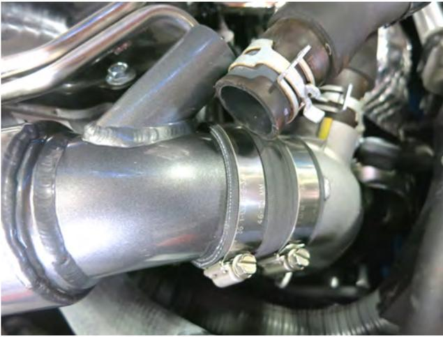
l. Tighten the hose clamp, holding the intake pipe to the coupler, to 30 in-lbs.
