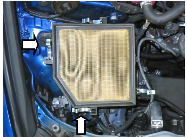
h. Remove the stock panel filter and the 2 M6 bolts holding the lower air box.
