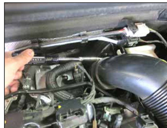
3. Loosen the hose clamp at the turbocharger and disengage the intake hose from the turbo inlet.
