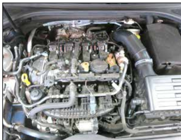
2. Remove the plastic engine cover by pulling up gently, releasing it from the rubber grommets.
