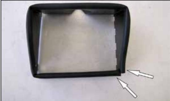
8. Install the provided bulb edge trim onto the top of the heat shield as shown.
