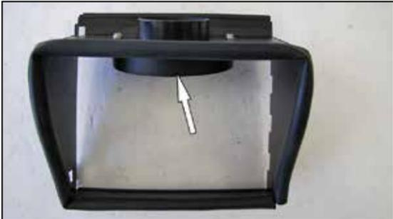
9. Install the filter adapter into the heat shield and secure with the provided hardware.
