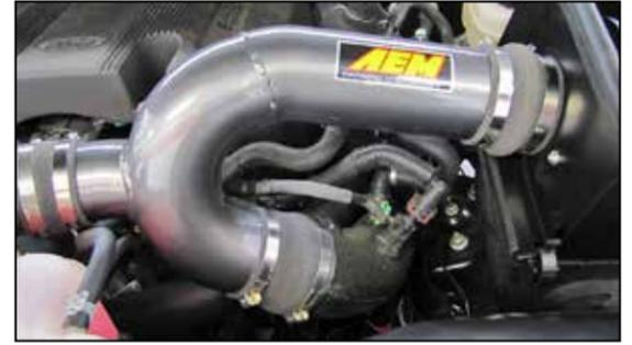
17. Install the AEM® intake tube into the couplers at the turbo inlet tubes and then into the coupler at the filter adapter, adjust the tubes for best fit and then secure with the provided hose clamps.
