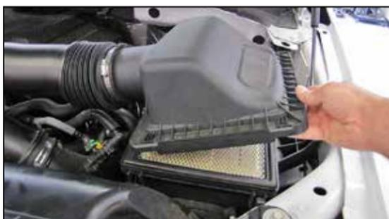
4. Release the locking clips that secure the upper air filter housing to the lower housing, then lift the upper housing and remove it from the vehicle. Remove the factory air filter from the vehicle.
