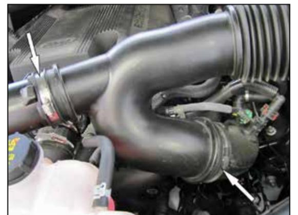
5. Loosen the two hose clamps that secure the factory intake tube to the turbo inlets and remove the factory tube from the vehicle.
