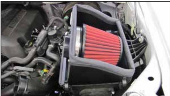
11. Install the heat shield/filter assembly onto the factory lower air filter housing and secure with the factory retaining clips.
