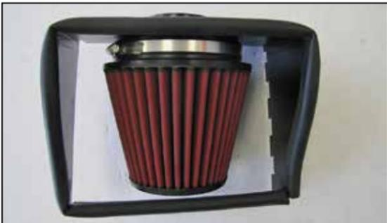
10. Install the air filter onto the filter adapter and secure with the provided hose clamp.
