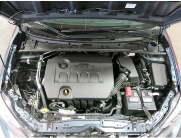
a. Pull up on engine cover to remove from rubber grommets.
