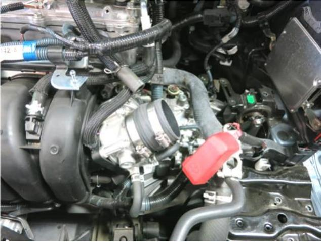
a. Install the coupler on the throttle body with the included hose clamps. Tighten the hose clamp on the throttle body side at this time.
