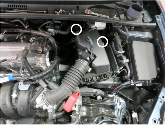
e. Loosen the clamp to the throttle body, unlatch the clips that hold the air box lid, and disconnect the PCV hose. Then remove the upper intake assembly.
