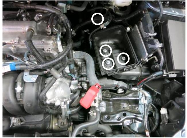
f. Unlatch the wiring harness from the air box, then remove the 3 bolts that hold the lower air box housing.
