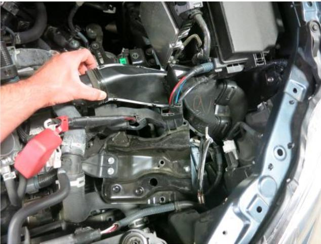
g. Maneuver the battery tray until there is clearance to remove the air scoop.
