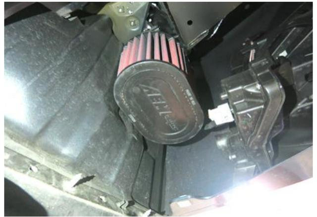
h. Install the air filter onto the tube. Be sure to have clearance around the filter before tightening the clamp.
