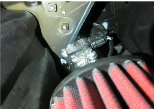
i. Connect the MAF harness extension to the MAF sensor. Then, reinstall the 2 bolts and push clip to secure the fender liner pulled back in step 3f.
