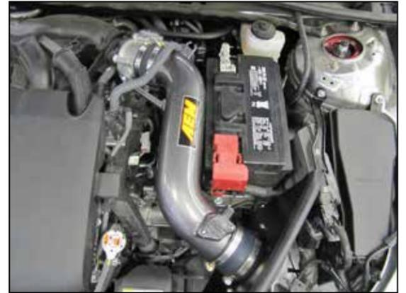
16. Install the AEM® intake tube into the Coupling hoses, adjust the tube for best fit and then secure with the provided hose clamps.
