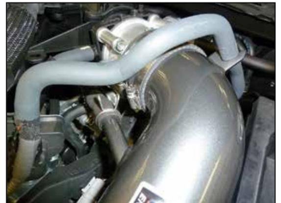
17. Connect the factory crank case vent line to the vent tube on the AEM® intake tube and secure the brake booster vacuum line to the intake tube as shown.
