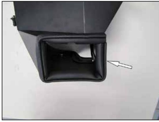
9. Install the side bulb edge trim onto the heat shield as shown.
