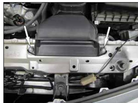
3. Remove the two bolts that secure the fresh air intake duct and then remove the duct from the vehicle.
