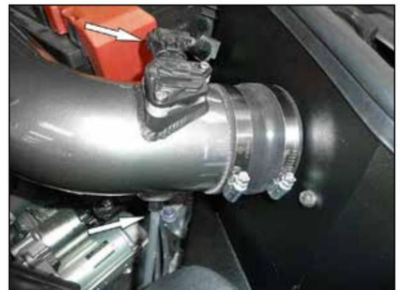
18. Connect the vacuum line to the AEM® intake tube and reconnect the mass air sensor electrical connection.
