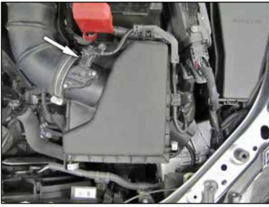
4. Disconnect the mass air sensor electrical connection and unclip the wiring harness from the air filter housing.
