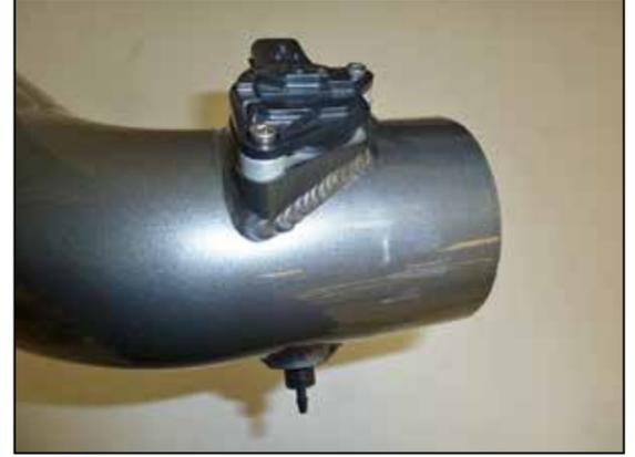
15. Remove the mass air sensor from the factory air filter housing and install it into the AEM® intake tube using the provided hardware. Install the provided vacuum fitting into the AEM® intake tube. **NOTE: Plastic NPT fittings are easy to cross thread. Install the vent fitting "hand" tight, then turn it two complete turns with a wrench.**
