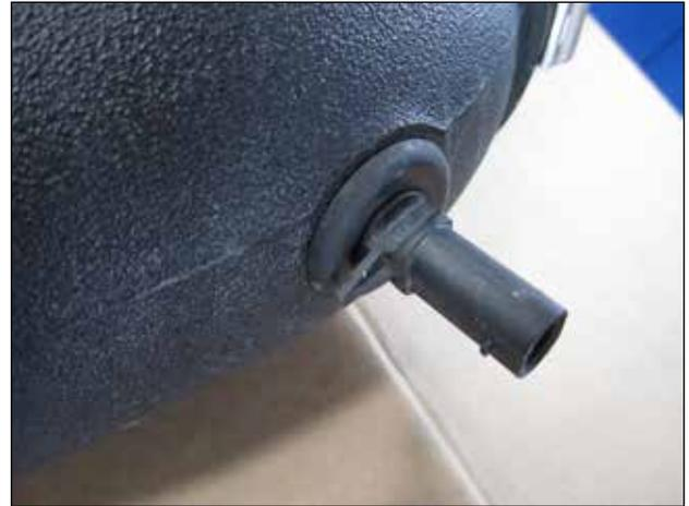
j. Install the stock IAT sensor into the grommet in the intake tube using glass cleaner for lubrication. Make sure the sensor O-ring is fully seated inside the grommet and orient the sensor as shown.
