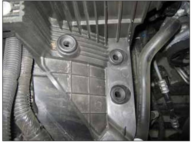
j. Make sure all 3 grommets are retained in the vehicle as shown.
