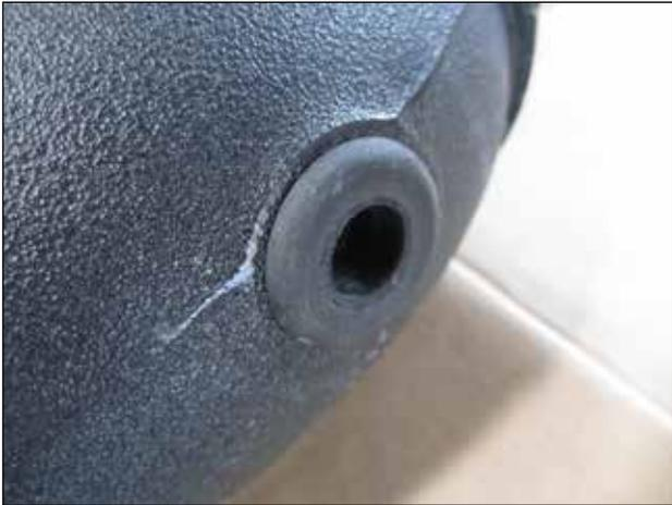
i. Install the other grommet into your new AEM intake tube as shown.
