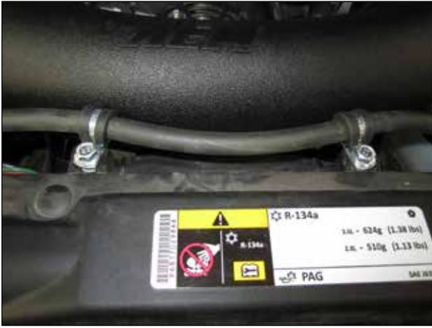
y. Install the 2 rubber insulated loop clamps over the stock coolant return hose. Install the two M6 X 20mm hex flanged bolts through the loop clamps and into the radiator upper cross member as shown.
