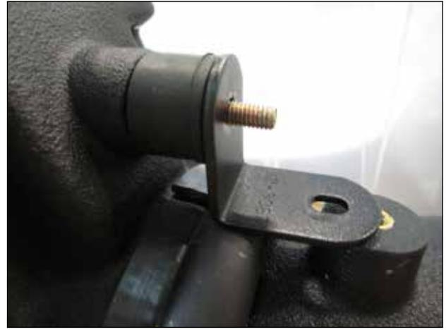
n. Install the "L" bracket onto rubber isolator mount as shown. The slotted hole should face the mounting boss on the intake tube.
