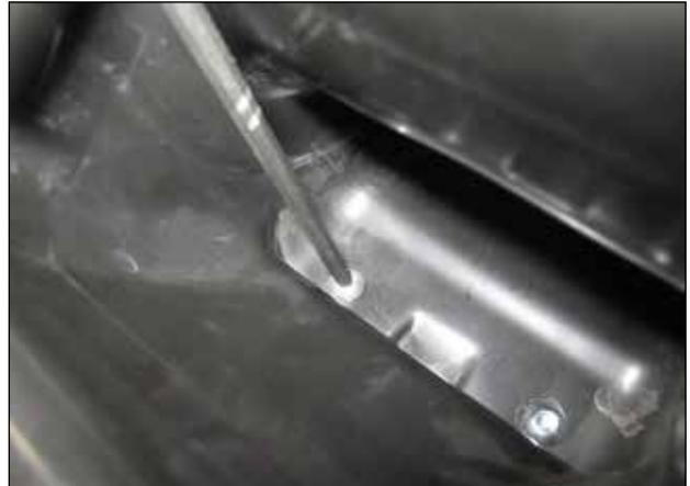
d. Hold the buttonhead bolts inside the inlet tube with an Allen key while tightening the M6 hex nuts on the outside with a 10mm wrench or socket.
