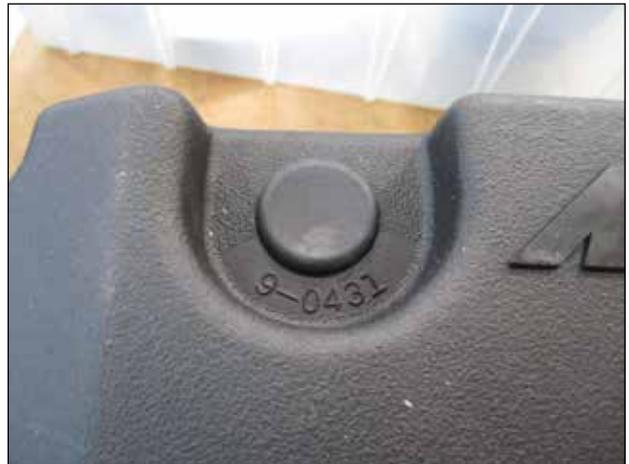
f. Install one plug into the hole in the AEM upper air box as shown.
