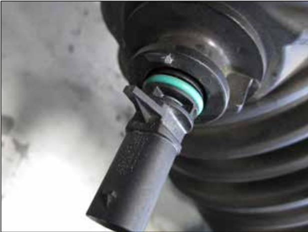
k. Remove the IAT (Intake Air Temperature) sensor from the stock intake tube by carefully lifting the locking tab and rotating the sensor, then pulling it from the tube. Save for use with your AEM intake.
