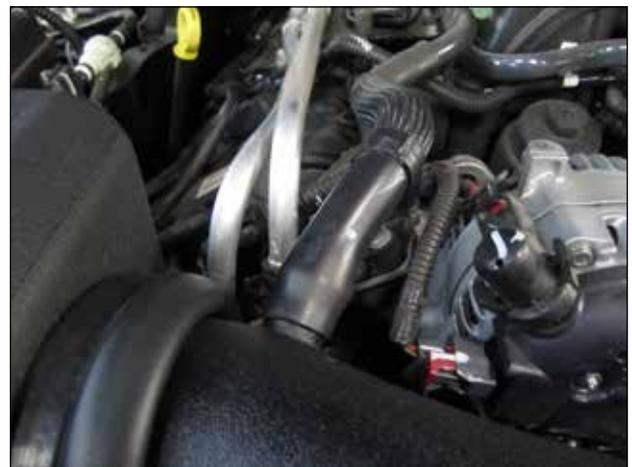
x. Connect the stock breather hose to the large port in new intake tube as shown.
