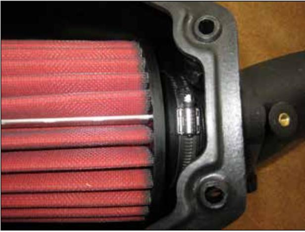
m. Rotate the intake tube back again until the mounting boss is aligned with the M6 rubber isolator mount as shown.
