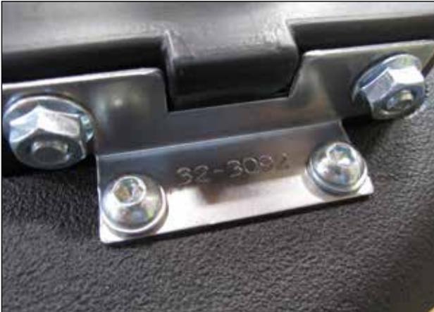
c. Mount the bracket onto the two button head bolts using two M6 hex nuts. Install the inlet tube into the lower airbox inlet and secure the bracket to the airbox using two split washers and two more M6 buttonhead bolts as shown.
