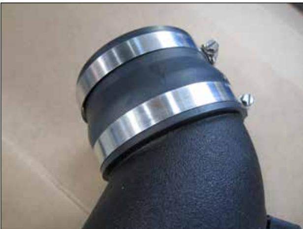
q. Install the rubber adapter onto the elbow end of the intake tube with a #56 hose clamp and tighten it. Loosely install the #52 hose clamp onto the smaller end.
