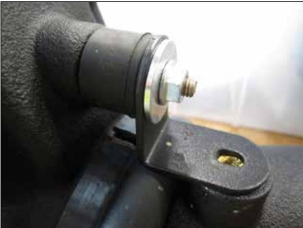
o. Install a flat washer and M6 hex nut onto the isolator mount stud as shown.
