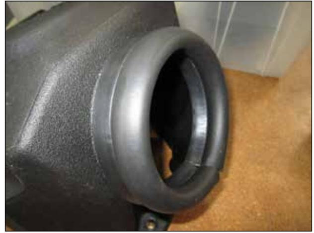
h. Install the rubber edge bulb seal around the edge of the upper airbox outlet as shown. Trim as needed.
