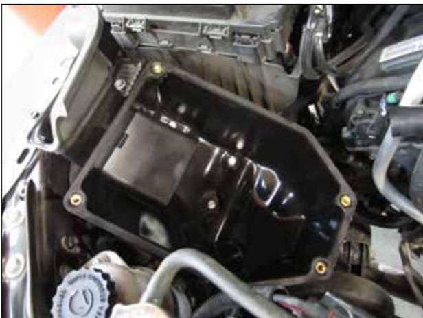
e. Install the lower airbox and inlet tube assembly onto the original airbox mounting grommets as shown.
