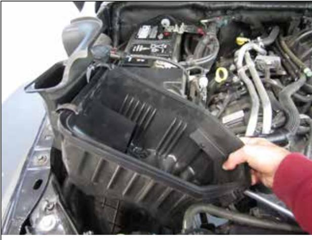
i. Remove the stock filter, and then remove the lower airbox and inlet tube from the engine bay by pulling up on the box to free it from the 3 rubber mounting grommets underneath it.
