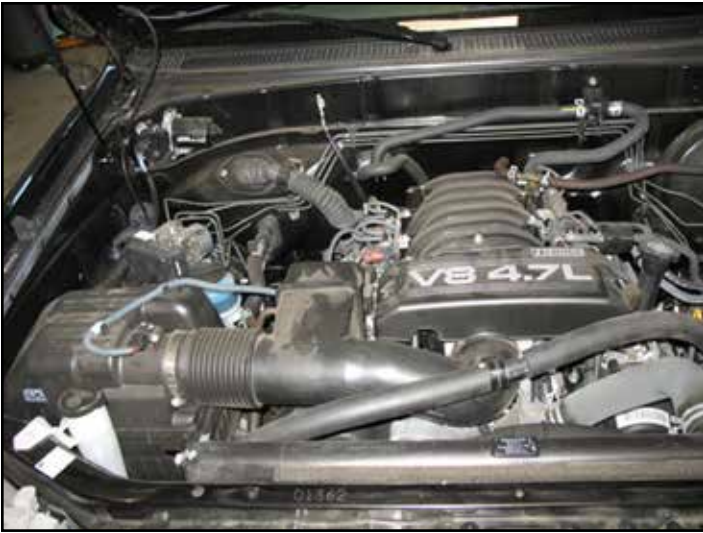
Factory intake system installed
