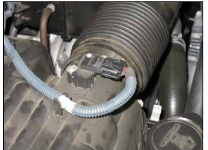
d. Disconnect the Mass Air Flow (MAF) harness from the MAF sensor.
