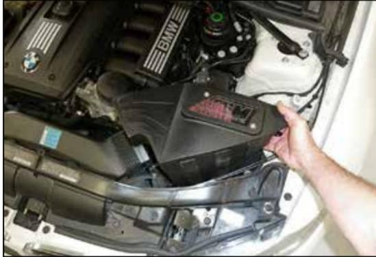
11. Install the AEM® filter housing assembly into the vehicle so that it sits on the factory bushings and the fresh air duct installs onto the AEM® air filter housing.
