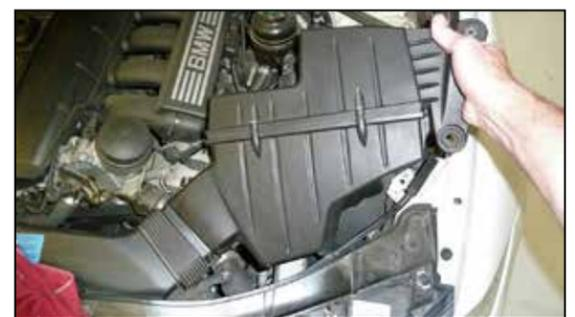
5. Remove the factory air filter housing from the vehicle.
