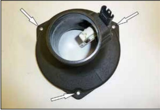
7. Install the provided spacers into the AEM® housing as shown.
