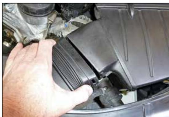
3. Disconnect the fresh air intake duct from the air filter housing.
