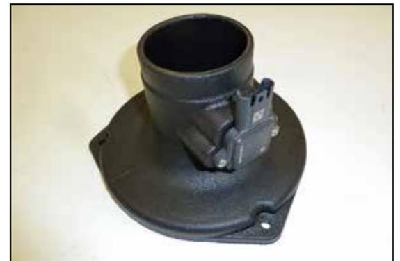
6. Remove the mass air sensor from the factory housing and install it into the AEM® housing and secure with the provided hardware.
