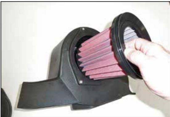
9. Install the AEM® air filter into the filter housing.
