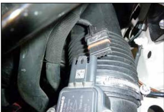
2. Disconnect the mass air sensor electrical connection. Loosen the hose clamp that secures the factory intake tube to the air filter housing.
