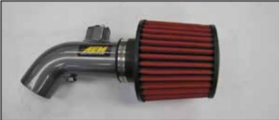
11. Install AEM® Dry Flow filter onto AEM® intake tube.
