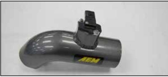
9. Remove the MAF sensor from the factory housing and install the sensor into the AEM® intake tube.
