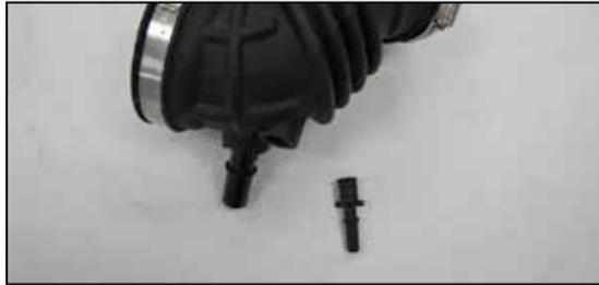
15. Move vent line fitting from stock intake tube.
