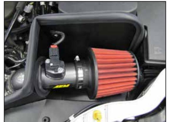
20. Route the MAF sensor wire harness through the heat shield cut out, then reconnect MAF sensor.
