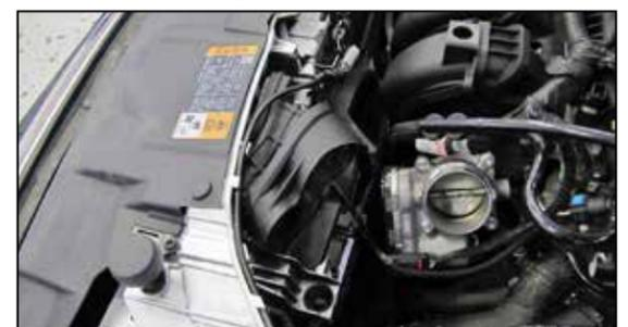
6. Pull on rubber intake duct to remove from vehicle.
