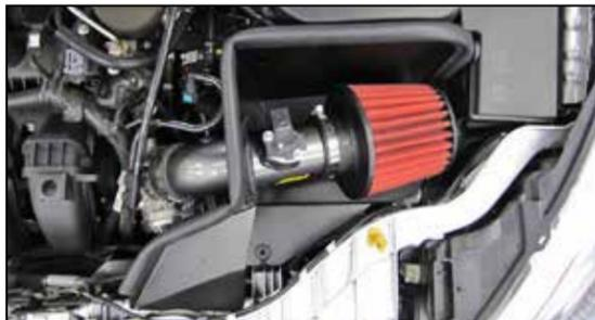
18. Install the AEM® intake system in the vehicle.
