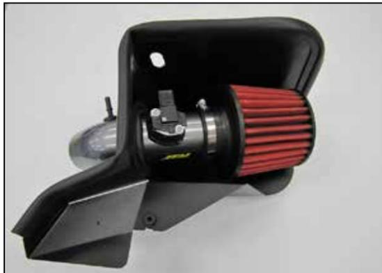
15. Install the factory vent fitting into the grommet as shown.
