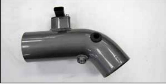
10. Install rubber grommet into AEM® intake tube.
