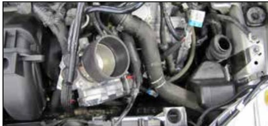
17. Install AEM® coupler on the throttle body as shown.
