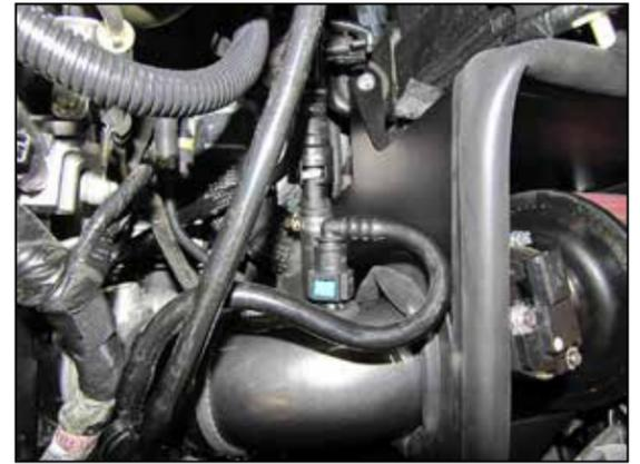
19. Install the supplied quick connect fitting onto NPT fitting, then reconnect crank case and vent line hose to the AEM® intake tube.
