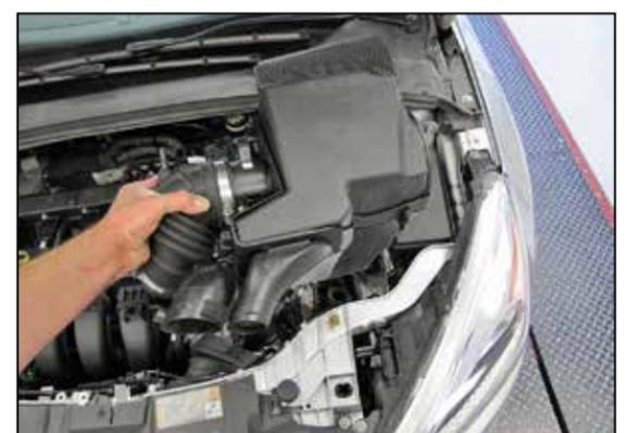
5. Pull up on intake system to release from push grommets to remove intake from vehicle.
