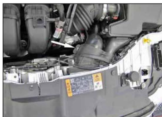
3. Release rubber strap for intake duct.
