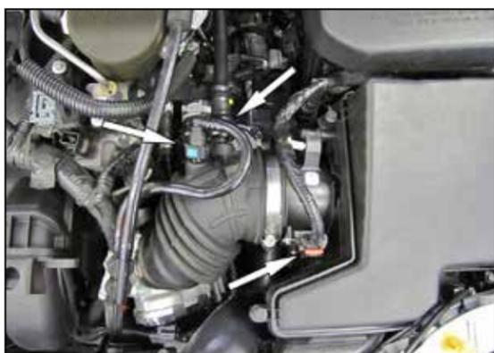
2. Disconnect MAF sensor, vent line, and crank case line from stock intake tube.
