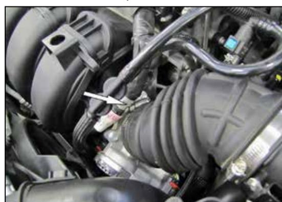
4. Loosen hose clamp on the throttle body.
