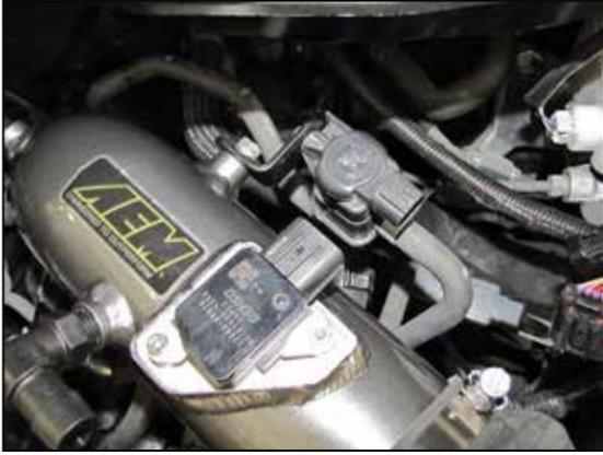
23. Secure the EVAP solenoid to the bracket installed onto the intake tube using the factory screw.
