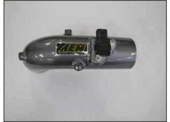
17. Remove the mass air sensor from the factory air filter housing and install it into the AEM® intake tube using the provided hardware.
