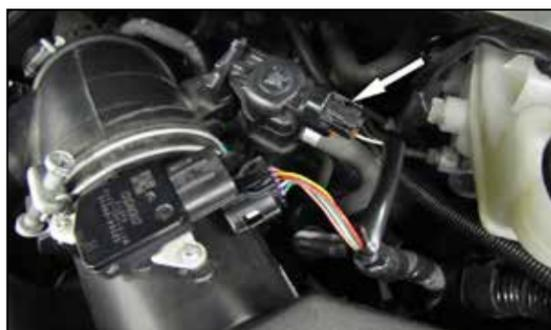
3. Disconnect the EVAP solenoid electrical connection.
