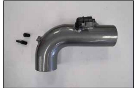
19. Install the EVAP vent fitting into the AEM® intake tube. On vehicles that are not equipped with the EVAP vent hose from the factory install the npt plug into the AEM® intake tube.
