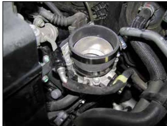
16. Install the provided coupler hose (5-302) into the throttle body and secure with the provided hose clamp.
