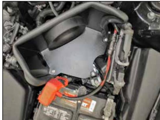
15. Install the heat shield into the vehicle so the fresh air duct slides over the fresh air tube on the heat shield. Secure the heat shield with the hardware provided.
