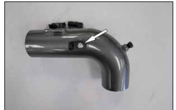
20. Install the EVAP solenoid mounting bracket (070066) onto the AEM® intake tube using the provided hardware.
