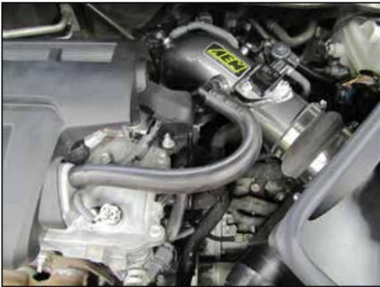
24. Install the provided crank case vent hose onto the fitting installed into the intake tube and onto the vent port on the valve cover.
