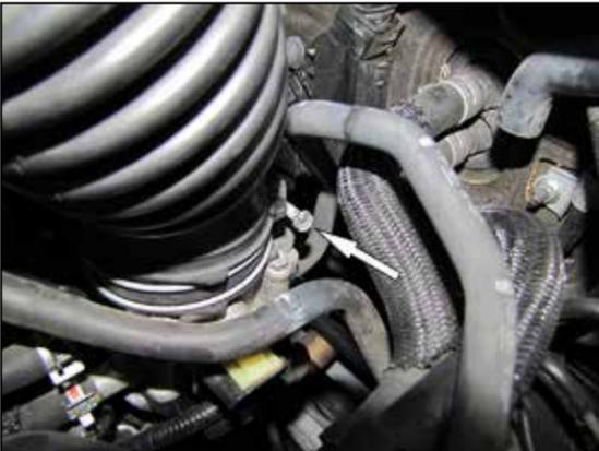
9. Loosen the hose clamp that secures the factory intake hose to the throttle body and then remove the intake hose from the vehicle.
