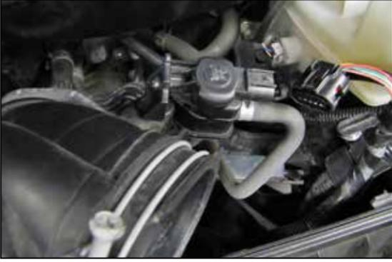
8. Unbolt the EVAP solenoid from the mounting bracket.
