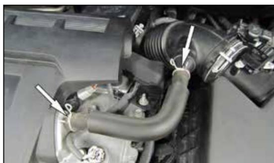
4. Release the spring clamps and remove the crank case vent line from the valve cover and intake tube.
