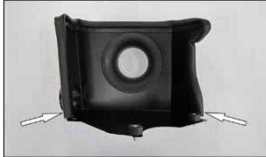
13. Install the provided edge trim onto the heat shield as shown.
