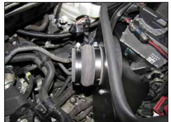
21. Install the provided hump coupler (084079) onto the filter adapter installed into the heat shield and secure with the provided hose clamp.
