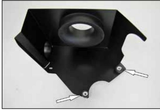
12. Install the provided rubber mounted studs onto the heat shield and secure with the provided hardware.
