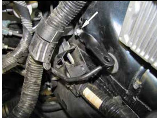
14. Install the heat shield mounting bracket (070702) onto the strut tower air filter housing mounting bracket location from step #10 using the hardware provided.
