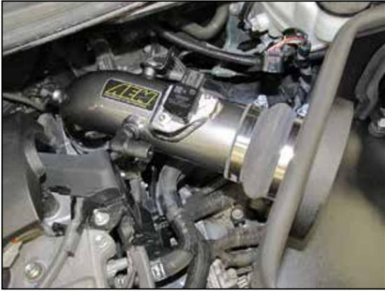
22. Install the AEM® intake tube into the coupler hoses, align for best fit and then secure with the provided hose clamps.
