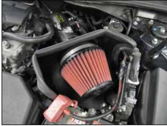
26. Install the AEM® air filter and secure with the provided hose clamp.
