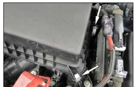
6. Release the two clips that secure the upper air filter housing, remove the upper air filter housing and factory air filter.
