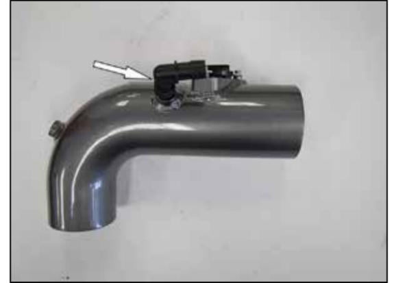
18. Install the 90° vent fitting into the AEM® intake tube as shown.
