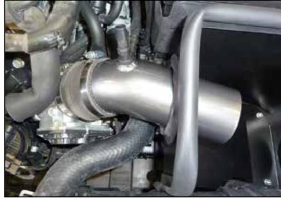
12. Install the AEM® tube through the heat shield and then into the coupler at the throttle body. Do not secure at this time.
