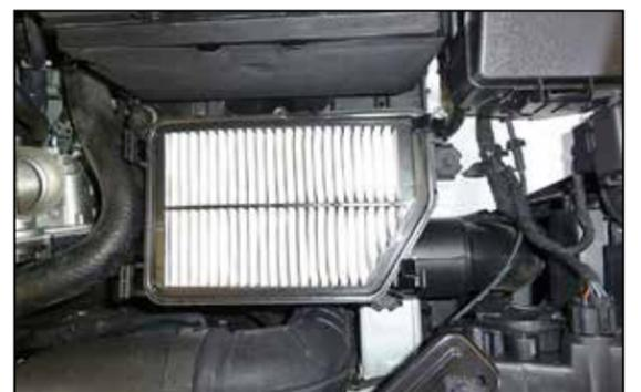
5. Remove the three bolts that secure the lower air filter housing to the inner fender and then remove the lower air filter housing from the vehicle. **NOTE: AEM recommends that customers do not discard factory air intake.**
