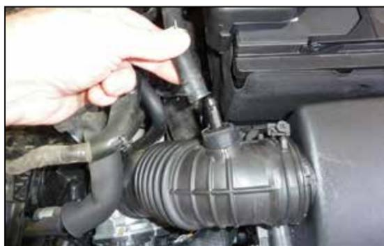
3. Disconnect the crank case vent hose from the factory intake tube.
