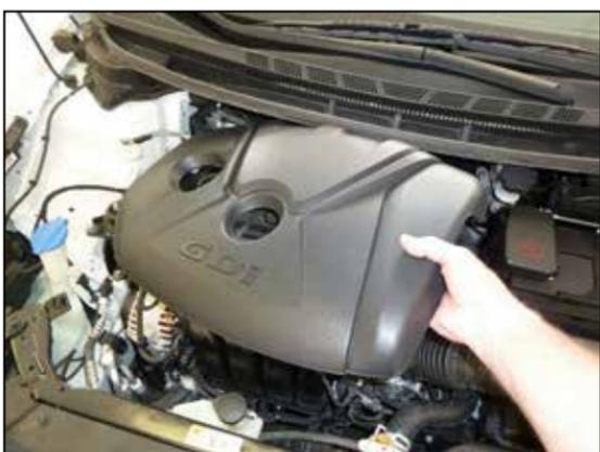
2. Lift the decorative engine cover up and remove it from the vehicle
