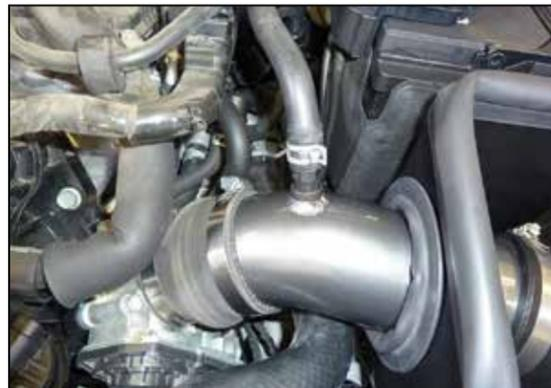
14. Connect the factory crank case vent hose to the fitting installed into the intake tube and secure with the factory clamp.
