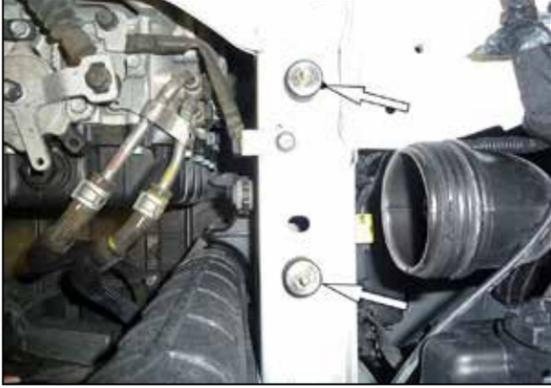
8. Install the two-provided rubber mounted studs onto the frame as shown.
