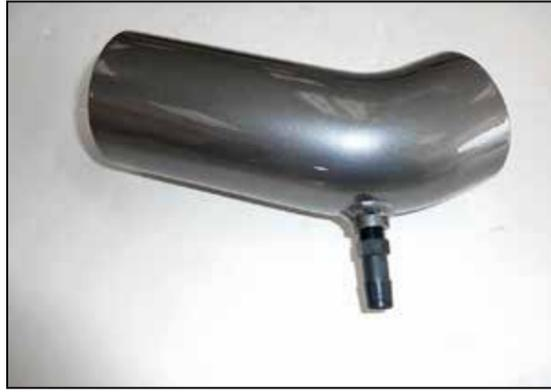
11. Install the provided vent fitting into the intake tube as shown.
