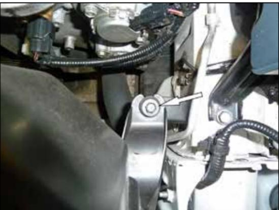
7. Remove the remaining air box mounting bolt then lift up the air box assembly and remove it from the vehicle.
