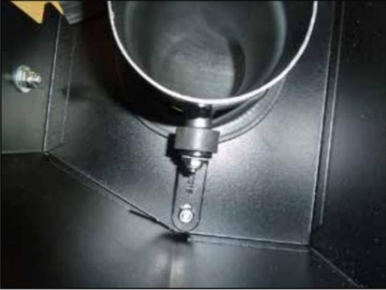
19. Rotate the tube down and install it into the coupling hose on the throttle body and install the mounting stud into the bracket. Secure the tube with the provided hose clamps and hardware and tighten the mounting bracket at this time.
