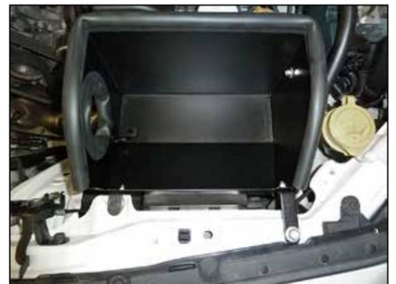
16. Set the heat shield into position on the core support and secure with the factory air box mounting bolts and to the previously installed bracket with the hardware provided.
