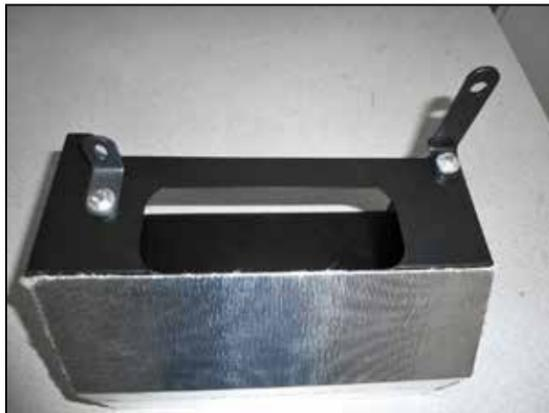
11. Install the provided "L" bracket (083170) onto the heat shield using the provided hardware. Install the provided "L" bracket (070066) onto the heat shield using the provided hardware.
