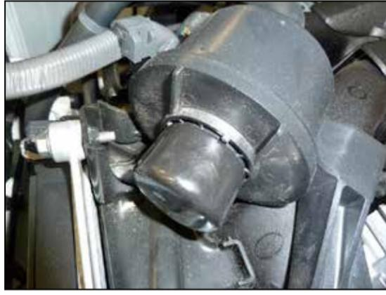
21. Install the provided caplug onto the sound drum.
