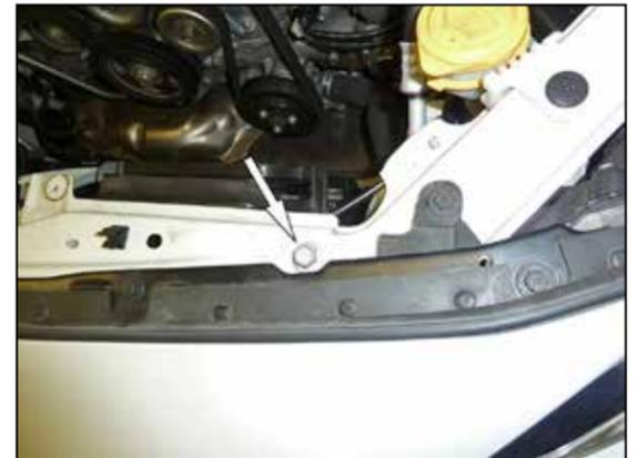
15. Remove the core support bolt shown.
