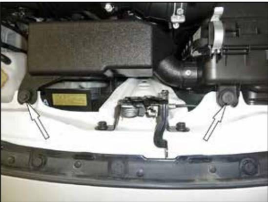
6. Remove the two bolts shown securing the resonator and air box to the core support.
