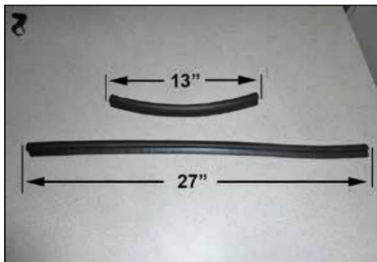
13. Cut the provided edge trim into two sections, one section is to be 27" long and the other section is to be 13" long.
