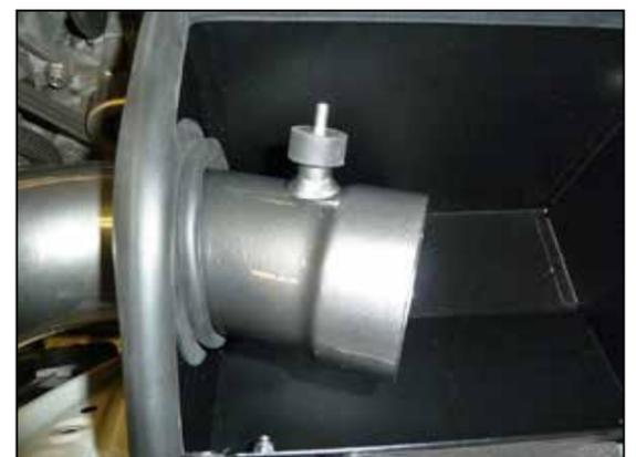
18. Install the tube through the heat shield and then install the provided rubber mounted stud onto the tube as shown.
