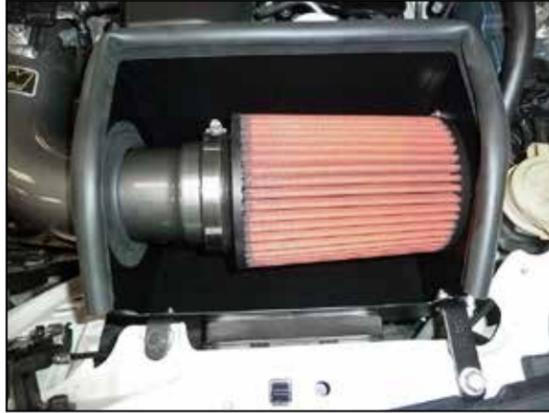
22. Install the air filter onto the AEM® intake tube and secure with the provided hose clamp.
