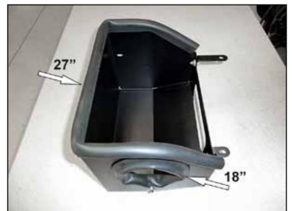
14. Install the 13" long section of edge trim into the hole of the heat shield as shown and then install the 27" long section of edge trim onto the top of the heat shield as shown.
