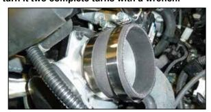
8. Install the provided coupler onto the throttle body and secure with the provided hose clamp.
