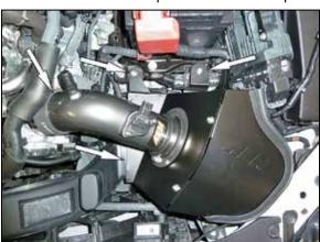
15. Install the complete intake assembly into the vehicle so the mounting studs engage with the factory air filter housing mounts, the intake tube engages the coupling hose and the fresh air intake duct inserts into the heat shield. Align the intake tube and then tighten the hose clamp that secures the intake tube.
