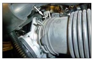
4. Release the spring clamp and disconnect the intake hose from the throttle body.
