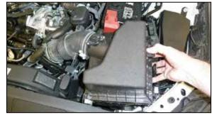
5. Lift up and remove the intake system from the
