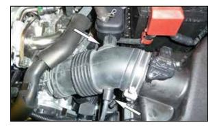
3. Disconnect the two vent lines from the intake tube.
