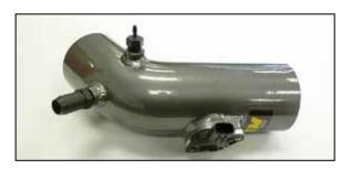
7. Install the two provided vents into the AEM® intake tube as shown.
