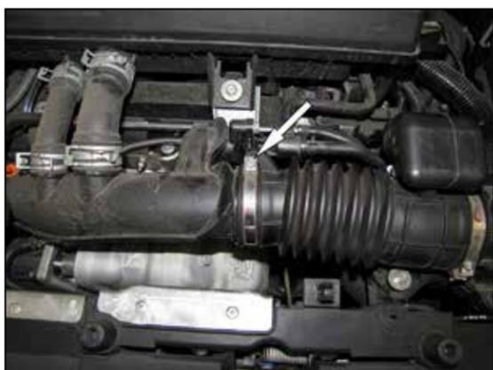
2. Loosen the hose clamp at the turbo inlet tube.
