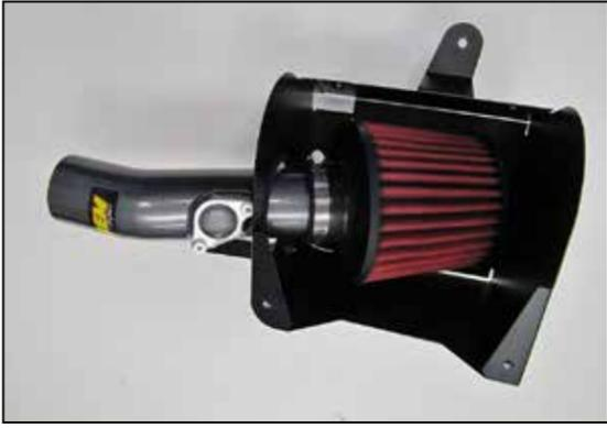
7. Set the air filter into the heat shield and then pass the intake tube through the heat shield and install the air filter onto the tube and secure with the provided hose clamp.
