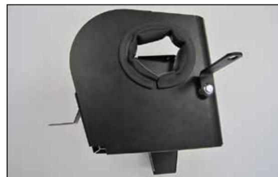
5. Install the provided edge trim into the hole of the heat shield as shown. Install the mounting bracket (010051A) onto the heat shield and secure with the provided hardware.
