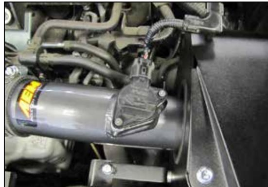
12. Reconnect the mass air sensor electrical connection.
