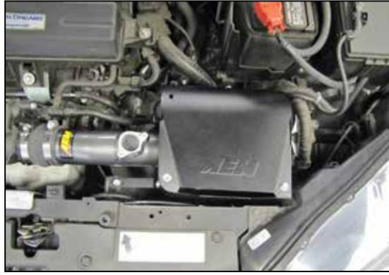
10. Install the complete assembly so the mounting stud protrudes into the mounting grommet, insert the intake tube into the coupler hose and align the mounting bracket. Secure the assembly with the hardware and hose clamp provided.
