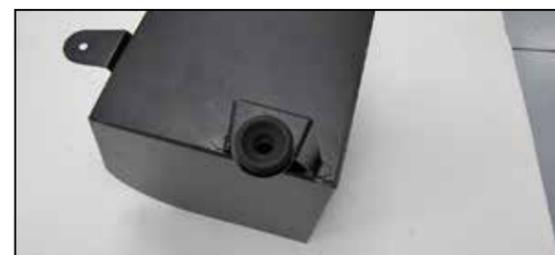
6. Remove the mounting grommet from the factory air filter housing and install it into the AEM® heat shield as shown.
