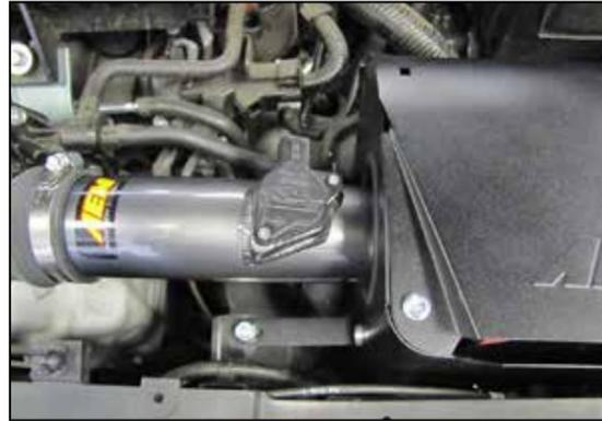
11. Remove the mass air sensor from the factory air filter housing and install the mass air sensor into the AEM® intake using the provided hardware.
