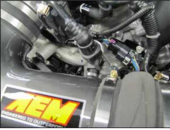
22. Connect the factory crank case vent line to the quick connect fitting installed into the AEM® intake tube.
