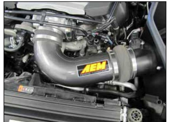
21. Install the AEM® intake tube into the hump coupler and then into the coupler at the throttle body, adjust the tube for best fit and then secure with the provided hose clamps.
