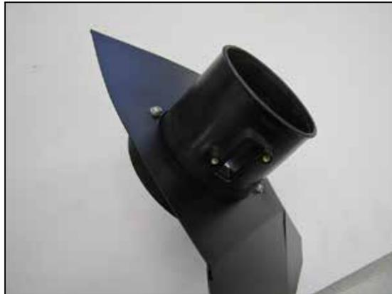
13. Install the provided mass air sensor housing into the provided heat shield and secure with the hardware provided.
