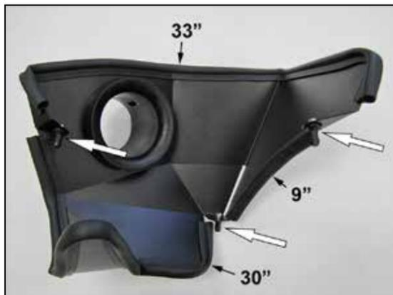
15. Install the edge trim onto the heat shield. Install the three provided mounting studs using the hardware provided.
