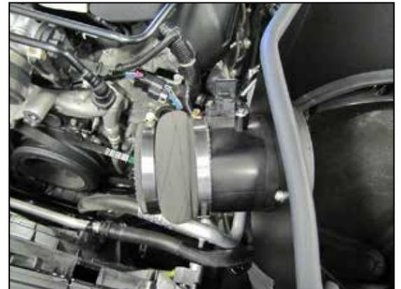
19. Install the provided hump coupler (08633) onto the mass air sensor housing and secure with the provided hose clamps.
