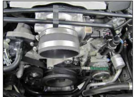
18. Install the provided coupler (08761) onto the throttle body and secure with the provided hose clamps.
