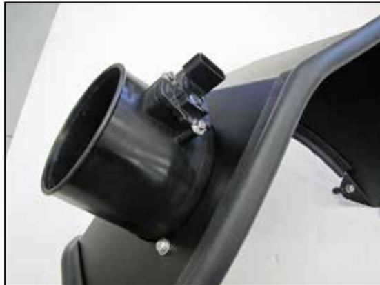
16. Remove the mass air sensor from the factory air filter housing and install it into the AEM® air filter housing using the provided hardware.
