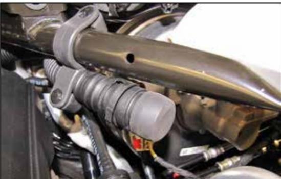
11. Install the cap plug assembly into the remaining factory sound tube quick connect fitting.
