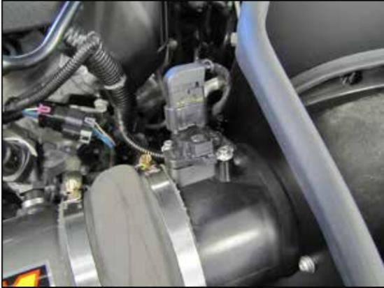
23. Reconnect the mass air sensor electrical connection.
