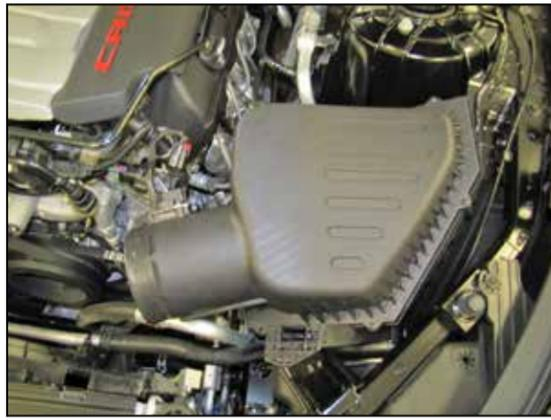
12. Remove the factory air filter housing from the vehicle.
