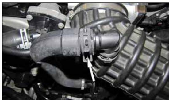
4. Release the spring clamp that secures the sound tube to the intake tube and then disconnect the sound tube.
