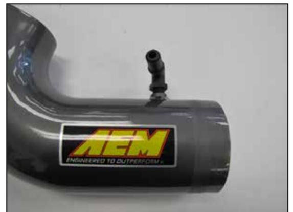
20. Install the 90° vent fitting into the AEM® intake tube as shown.
