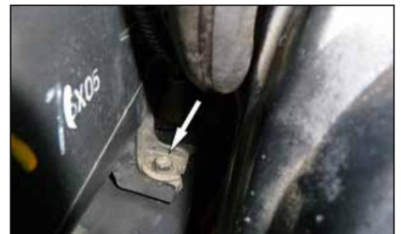
5. Remove the bolt that secures the air filter housing to the frame rail.
