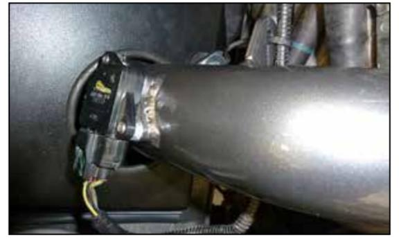
16. Reconnect the mass air sensor electrical connection and secure the wiring harness with the provided tie wrap to the bracket on the intake tube.
