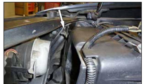
6. Remove the nut that secures mounting bracket to the air filter housing and remove housing from the vehicle.
