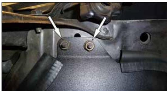
14. Secure the heat shield to the inner fender using the factory nuts removed earlier.
