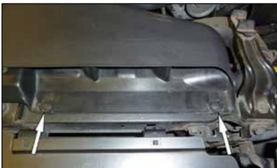
2. Remove the two plastic retaining clips that secure the fresh air intake duct.
