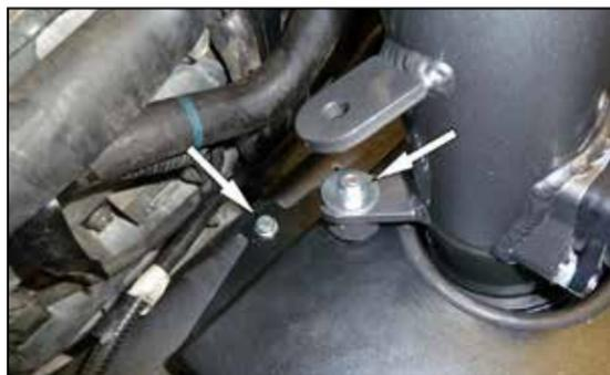
15. Secure the heat shield to the frame rail using the provided hardware. Align the intake tube for best fitment, secure it to the rubber mounted stud using the provided hardware and tighten the hose clamp.
