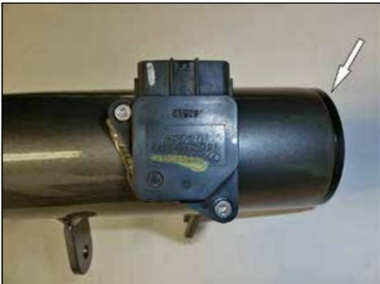
10. Remove the mass air sensor from the factory air filter housing and install it into the AEM intake tube and secure with the provided hardware. Install the provided venturi sleeve into the intake tube so that the slot goes around the mass air sensor.
