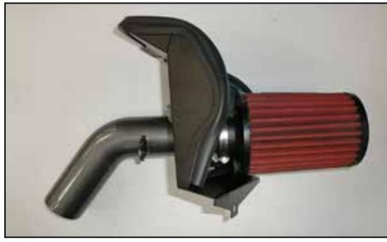
11. Install the heat shield assembly onto the intake tube and secure with the provided hardware. Install the air filter onto the intake tube and secure with the provided hose clamp.
