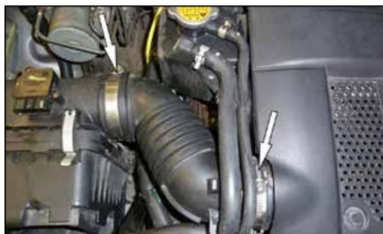
4. Loosen the hose clamps that secure the factory intake tube and then remove the intake tube from the vehicle.
