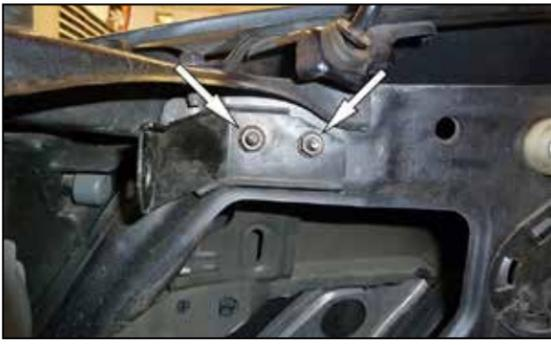
7. Remove the two nuts that secure the filter housing mounting bracket to the inner fender and then remove the mounting bracket from the vehicle.
