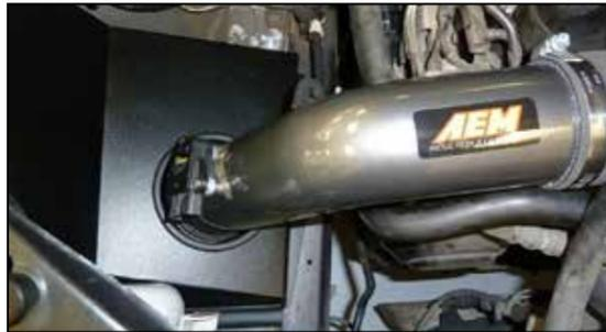
13. Install the intake kit into the vehicle so the intake tube goes into the coupler hose and the studs on the inner fender protrude through the holes in the heat shield.
