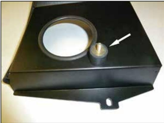
9. Install the provided small edge trim into the hole of the heat shield and then install the rubber mounted stud onto the heat shield and secure with the provided hardware.
