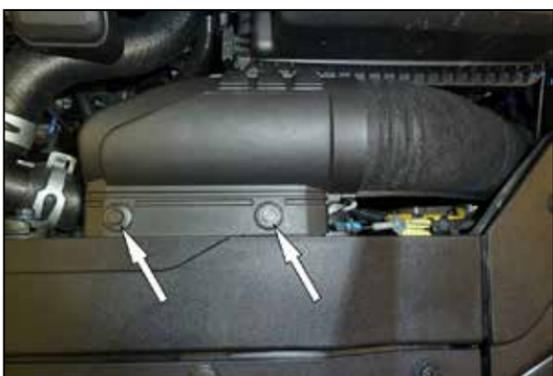
2. Remove the two push pins that secure the fresh air intake duct and then remove the fresh air intake duct from the vehicle.
