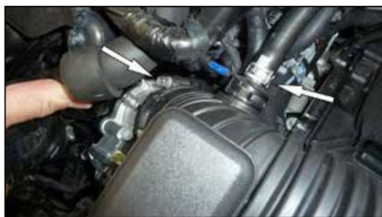
3. Loosen the clamp that secures the factory intake hose to the throttle body. Release the spring clamp that secures the crank case vent line and disconnect the crank case vent from the factory intake hose.
