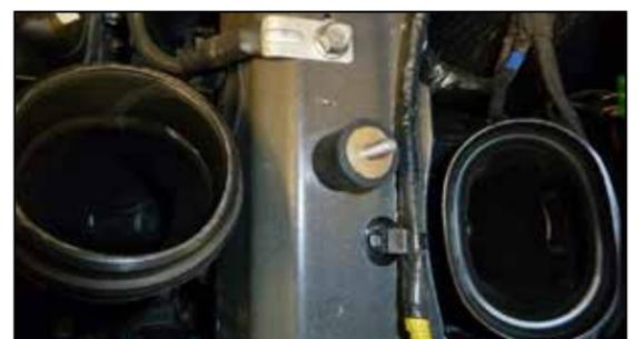
6. Install the provided rubber mounted stud onto the frame rail as shown.
