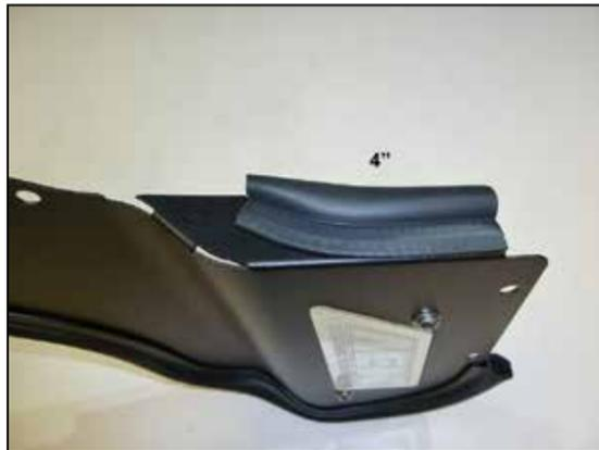
14. Install the remaining edge trim onto the heat shield as shown.
