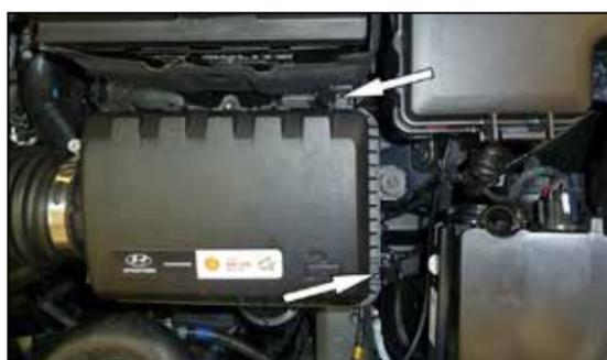
4. Release the two upper air filter housing spring clips and then remove the upper housing, intake hose and filter from the vehicle.
