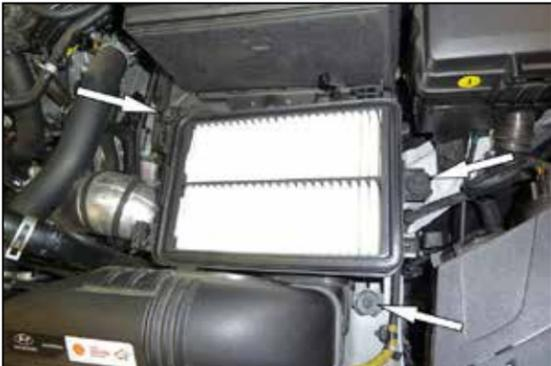
7. Remove the three bolts that secure the lower air filter housing and then remove the lower housing and fresh air duct from the vehicle.
