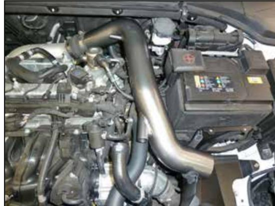
13. Install the intake tube into the coupler and onto the heat shield, adjust for best fit and then secure with the provided hardware.
