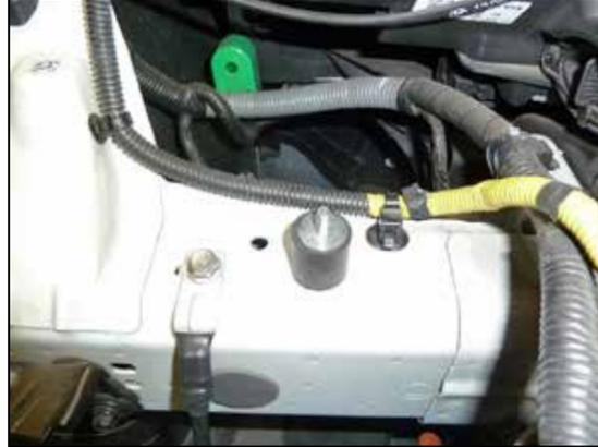
10. Install the provided rubber mounted stud into the air filter housing mounting location on the frame rail as shown.
