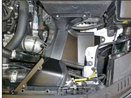
11. Install the heat shield into the vehicle and secure with the hardware provided.
