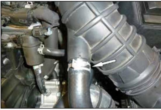
4. Release the spring clamp that secures the BOV hose to the intake tube and then disconnect the BOV hose.
