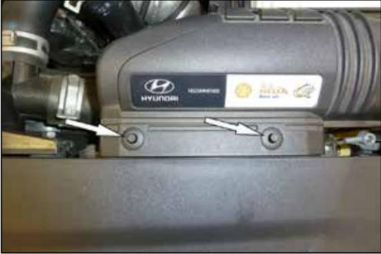
6. Push in the center of the fresh air intake duct retaining pins and then remove the pins from the vehicle.
