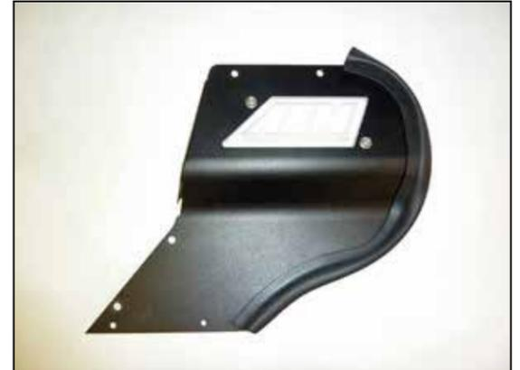
16. Install the AEM® window into the heat shield lid and secure with the provided hardware. Install the long edge trim onto the heat shield lid.
