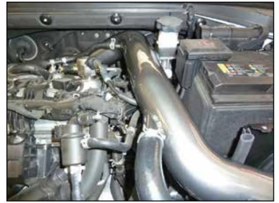
14. Connect the PCV hose and BOV hose to the AEM® intake tube and secure with the factory spring clamps.
