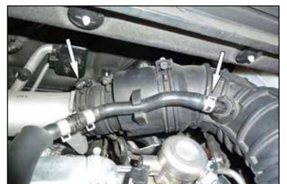
3. Loosen the clamp that secures the factory intake tube to the turbo inlet pipe. Release the spring clamp that secures the PCV hose to the intake tube and then disconnect the PCV hose.
