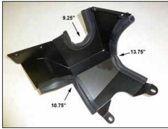
9. Install three of the edge trims onto the heat shield as shown.
