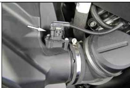
2. Disconnect the inlet air temperature sensor electrical connection and loosen the hose clamp that secures the factory intake tube to the air filter housing. Pull up the air filter housing to release it from the mounting grommets and remove it from the vehicle. **NOTE: On models that are equipped with a strut tower brace use a E14 reverse TORX socket or a 7/16" 12 point socket to remove the bolts that secure the strut brace.**
