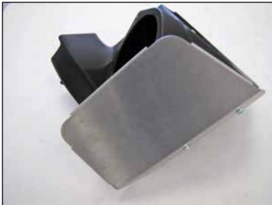
7. Install the provided heat shield onto the rubber mounted studs using the provided hardware.
