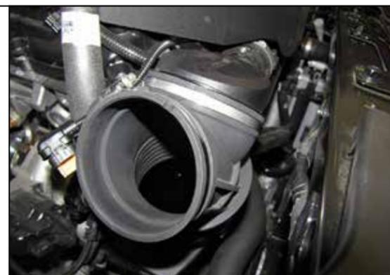
3. Loosen the hose clamp that secures the intake tube to the turbo inlet and then remove the intake hose from the vehicle. **NOTE: AEM recommends that customers do not discard factory air intake.**
