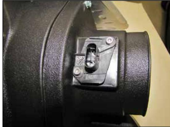
10. Remove the intel air temperature sensor from the factory housing and install it into the AEM® housing using the provided hardware.
