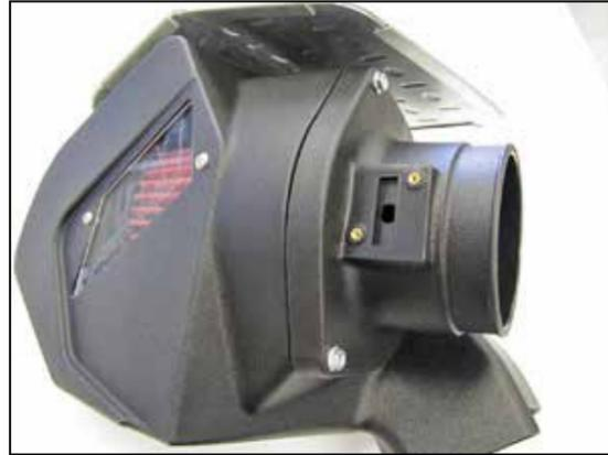
9. Install the temperature sensor housing onto the air filter housing and secure with the provided hardware.
