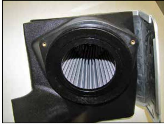
8. Install AEM® air filter into the filter housing as shown.
