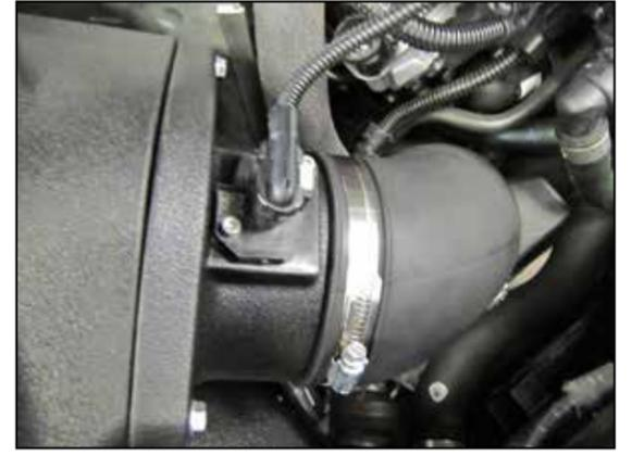
12. Reconnect the inlet air temperature sensor electrical connection.
