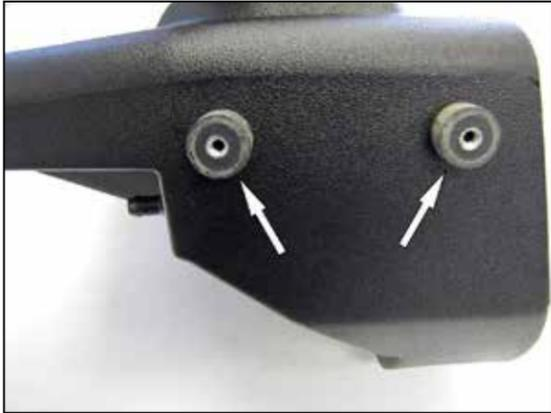
6. Install the two provided rubber mounted studs onto the AEM® air filter housing using the provided hardware.
