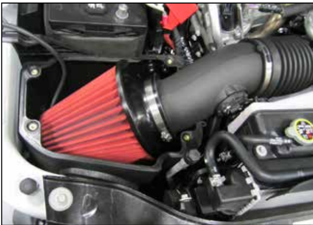
r. Plug in the MAF sensor. Align the AEM® air filter and intake tube for best fitment, then tighten the hose clamps.
