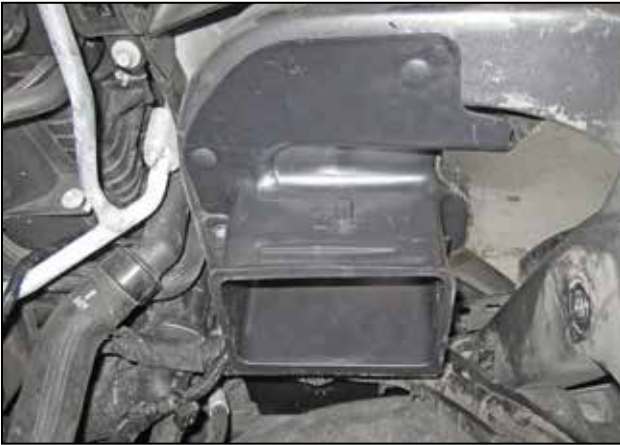
m. Remove the OEM air box bracket.
