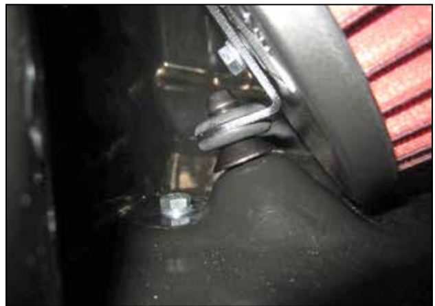
q. Install the intake assembly, ensuring the large grommet attached to the air box's bracket engages the barb on the inside of the AEM® air box.
