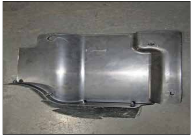
r. Using a hack saw or other suitable cutting tool, cut the OEM inlet duct on the line marked previously.
