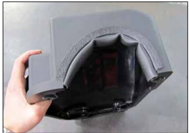
s. Install the edge trim (8-4010) on the side hole of the AEM® air box lid (9-0409).
