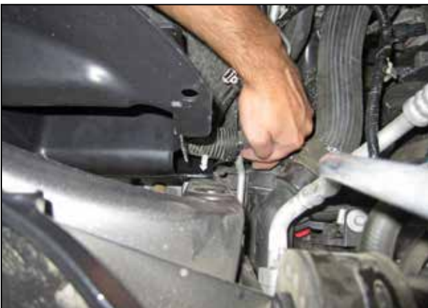
o. Disengage the plastic wire harness clip toward the bottom of the OEM inlet duct.
