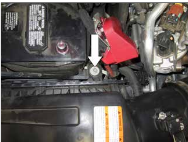
c. Remove the bolt securing the air box in place.
