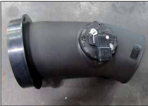
n. Install the filter adapter (5-1068) as shown by stretching it over the flared out end of the AEM® tube (9-0400).
