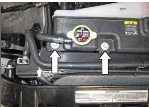
u. Loosen both screws securing the coolant reservoir to the radiator.
