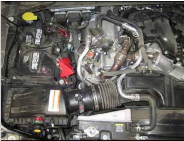
a. Loosen the hose clamp at the air box neck.
