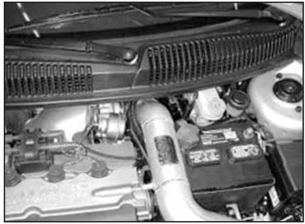
g. Attach the other end of the silicon coupler to the turbo inlet. Line up the bracket on the inlet pipe to the rubber mount. Secure the hose clamp.
