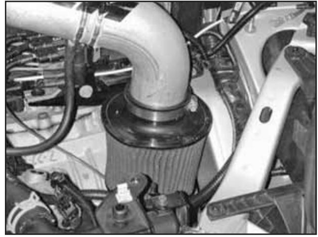
p. Attach filter element. Secure with provided hose clamp.
