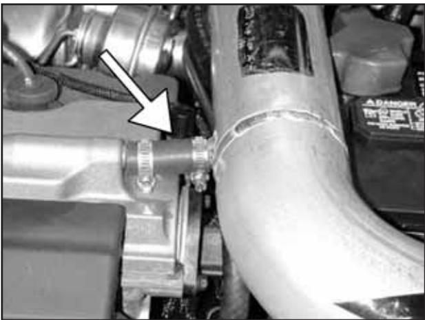
h. Attach breather hose from the crankcase to the inlet pipe. Secure with provided hose clamps. Make sure the nipple on the valve cover and pipe are fully inserted into the hose.
