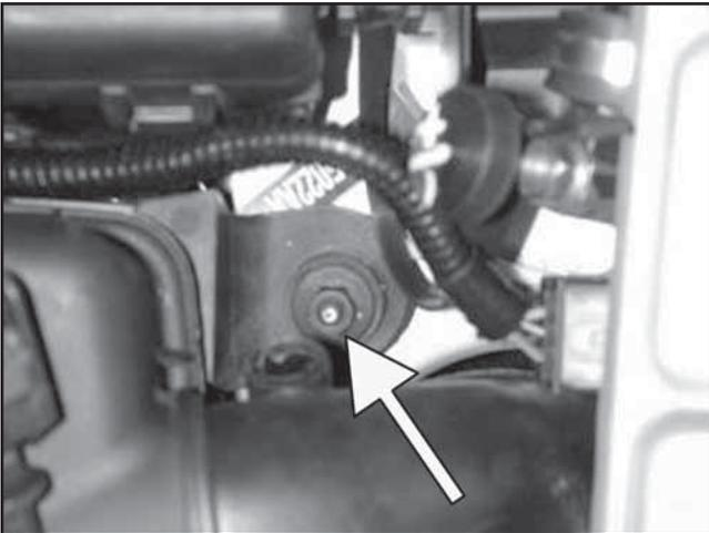
g. Loosen and remove nut holding down the air box. This nut is located by the vacant hole left by the IAT sensor.
