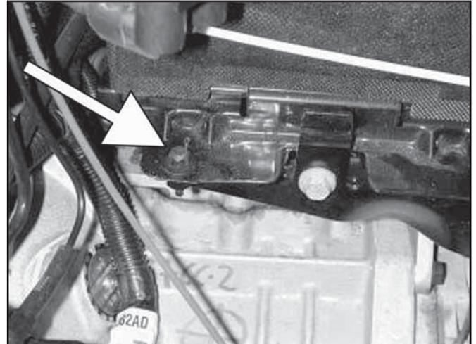
b. Loosen and remove the bolt on the right side of the battery bracket.
