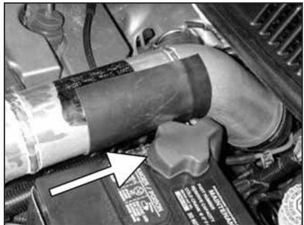
i. Make sure neoprene rubber adhesive clears the positive battery terminal. Make sure the (+) post protector on the battery is not damaged, cracked or melted. If any of the conditions exist, you must replace before completing the installation of the AEM® intake system. Failure to not follow these instructions will void warranty.
