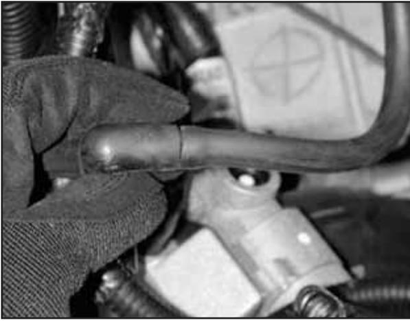
o. Insert vacuum fitting into the vacuum cap left from the installation Step 2d.
