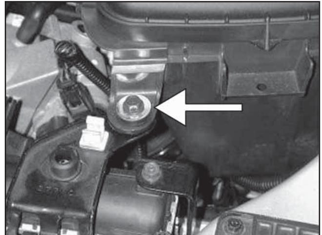
h. Remove bolt holding down the air box to the radiator support.
