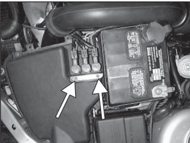
i. Remove the 2 bolts holding down the vacuum assembly to the air box.
