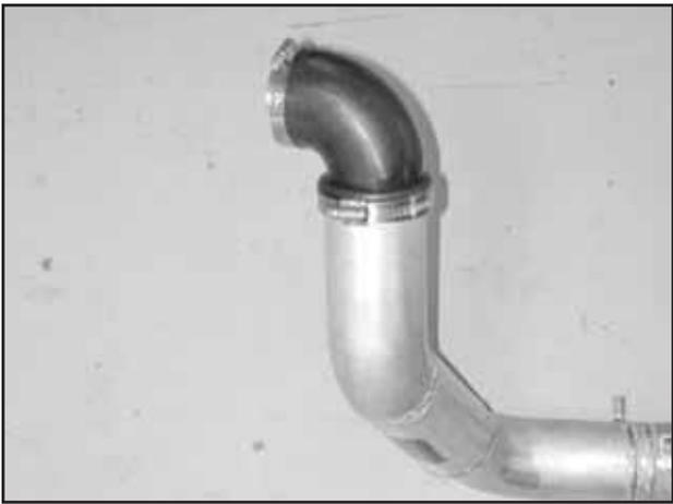
f. Attach the 3" side of the silicon elbow to the inlet pipe. Secure elbow to the inlet pipe. The open end connects to the turbo inlet which sits horizontal.
