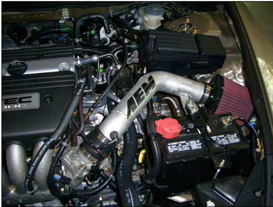
AEM® intake system installed
