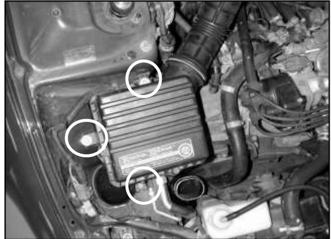
f. Remove the three air box mounting bolts and remove the factory air intake system from the car.
