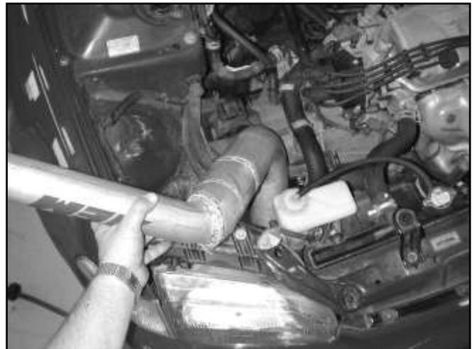
e. Insert the intake pipe into the engine bay as shown. Position the intake pipe so the 3.5" end is in the area behind the front bumper where the resonator was located.
