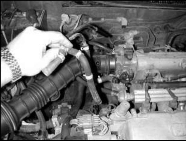
c. Detach the PCV hose from the fitting on the valve cover. Remove the hose assembly from the car.
