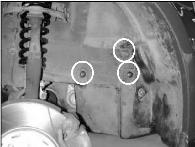
g. After removing the front right wheel, remove the fender liner fasteners shown in the picture.
