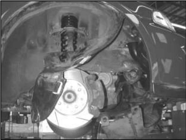
i. Tuck the fender liner out of the way behind the brake rotor.
