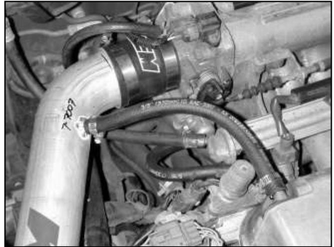
g. Insert the 2.5" end of the pipe into the silicone coupler on the throttle body. Use the #40 hose clamps on the coupler. Install the 3/8" ID hose from the valve cover breather fitting to the nipple on the intake pipe. Use the 1" hose clamps to secure it in place.
