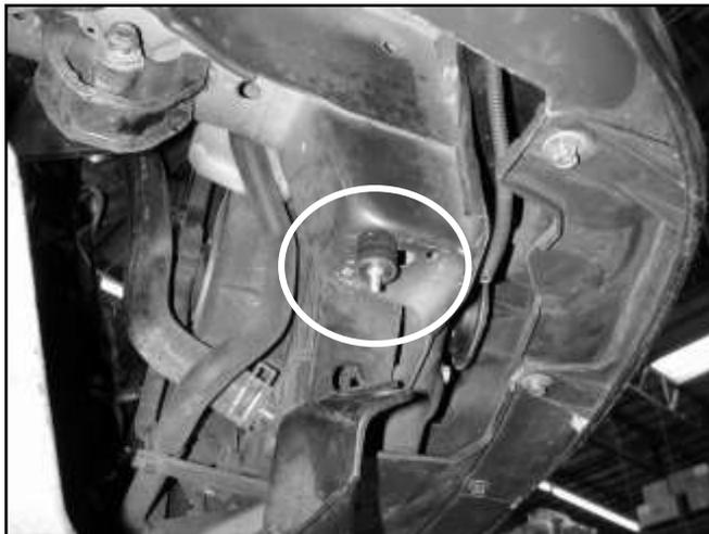
d. Thread the rubber mount into the hole on the bottom of the vehicle. (Hole that is exposed from the intake resonator removal during step 2j).
