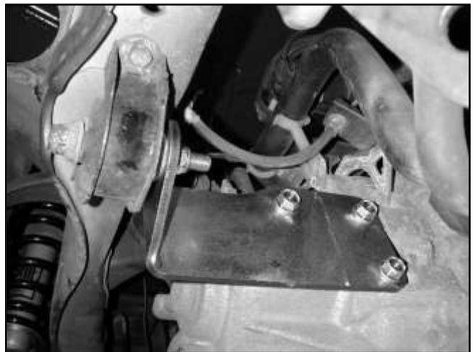
d. Using the supplied bolts, install the AEM® engine mount on the transmission; torque the bolts to 61 ft-lb. Then replace the factory washer and nut on the mounting stud.
