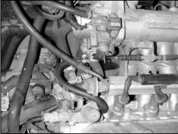
b. Install the 5/16" ID hose, and two 3/4" hose clamps, in place of the hose assembly removed in Section 2a & 2b.
