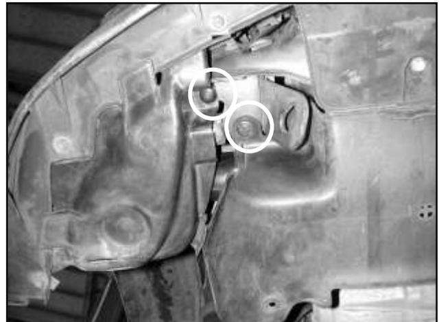
h. From underneath the car, remove the splash guard fasteners shown in the picture.
