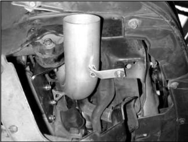
f. Line up the intake pipe support tab with the rubber mount. Install the rubber mount assembly as shown in the diagram below.
