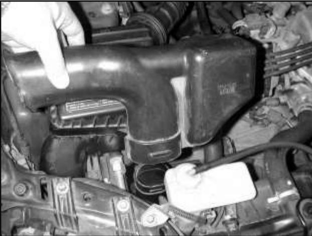
e. Remove the air intake snorkel by pulling it straight up until it unsnaps.
