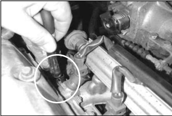
a. Remove the water hose on the left of injector #4 by loosening the hose clamp and sliding the water hose upward. Be prepared to catch any coolant that spills out with a rag.
