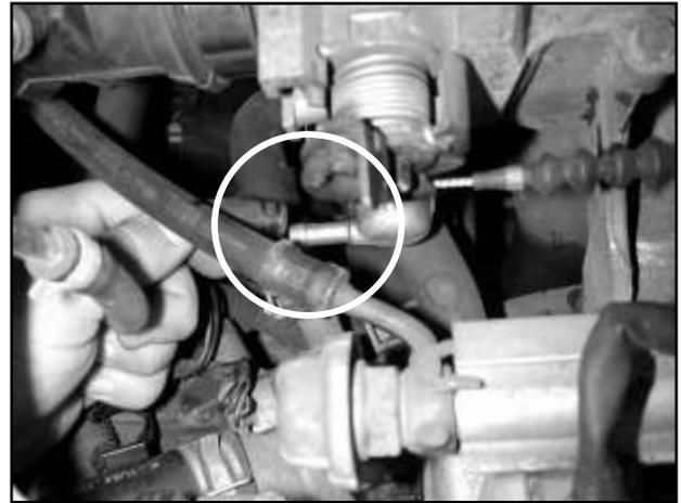
b. Remove the other end of the water hose from the fitting underneath the throttle body.
