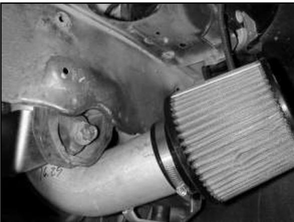
h. Install the air filter on the end of the intake pipe. Make sure the air filter is fully seated on the end of the pipe. Secure it in place with the supplied hose clamp.
