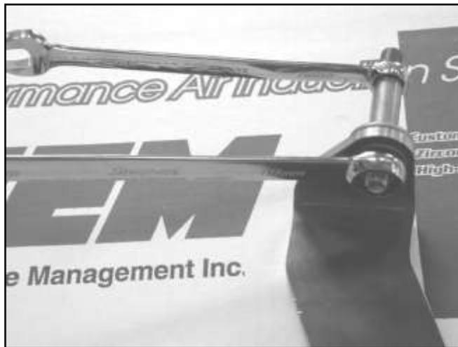
c. Install the factory mounting stud from step b on the supplied engine mount bracket, using the nylock nut and washer provided.
