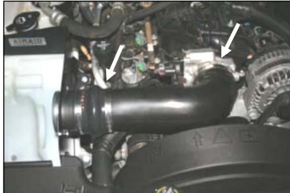
11. Insert the Airaid Intake Tube (#2) into the hump hose first. Then, insert the throttle body end of the tube into the coupler. Adjust for fit, and tighten the clamps.
