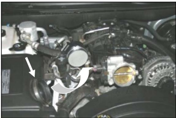
**4.** Loosen the clamp holding the Mass Air Flow (MAF) sensor to the factory airbox lid. Remove the complete factory intake and breather tube. Remove the MAF sensor from the lid (*do not disconnect it*), and then set it aside.
