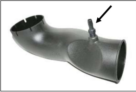
10. Insert one 1/4" NPT x 3/8" barbed fitting (#15) into the Airaid Intake Tube (#2).
