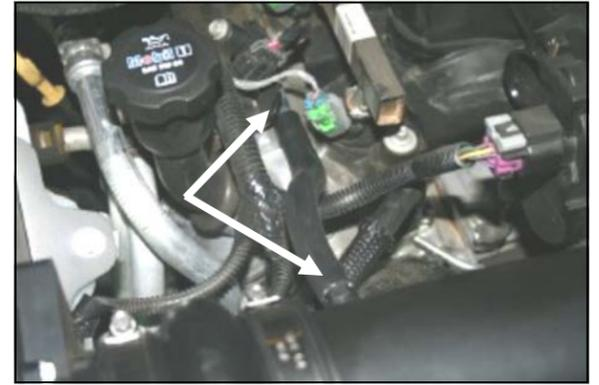
12. Slide one end of the 3/8" x 8" breather hose (#16) over the barbed fitting in the Airaid Intake tube. Slide the other end of the breather hose onto the metal tube on the engine.
