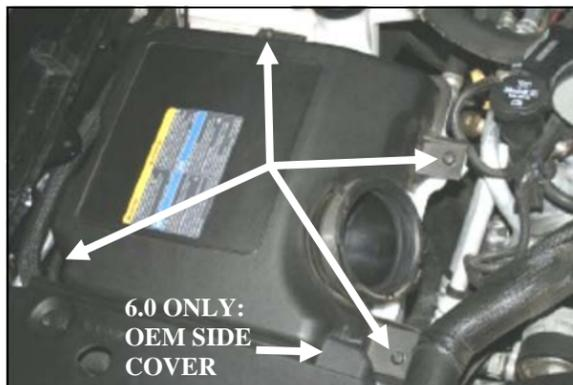
**5. 6.0 Liter Only:** Using a flat blade screwdriver, gently pry the plastic retaining clip from the OEM side cover.
