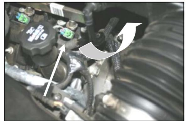
**3.** Slide the factory breather hose off of the metal tube on the engine.
