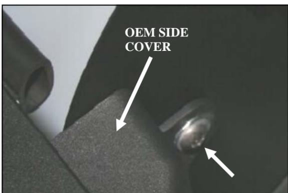
**7. 6.0 Liter Only:** Insert one 1/4 - 20 x 1/2" button head bolt (#8) and 1/4" flat washer (#9) through the hole in the OEM side cover, and through the hole in the panel. Secure using one 1/4 - 20 serrated nut (#10).
