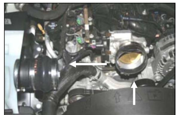
**9.** Slide the silicone hump hose (#4), and two #56 hose clamps (#14) onto the MAF sensor. Slide the coupler (#5) and one #68 hose clamp onto the throttle body. Tighten only the clamp on the MAF sensor for now.
