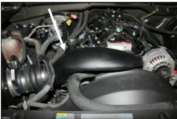
11. Install the small end of the intake tube into the hump hose first and then rotate it slightly to slide the other end onto the throttlebody. Adjust for fit, and then tighten all three hose clamps.
