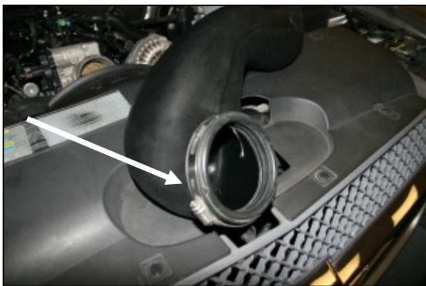
10. Install the provided coupler with clamp (#6) onto the large end of the Airaid Intake tube (#2). Do not tighten the clamp at this time.
