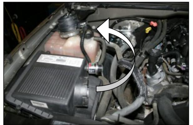
**3.** Remove the factory intake tube from the vehicle. Next, remove the MAF sensor and coupler from the factory airbox and set them out of the way without disconnecting the wiring harness.
