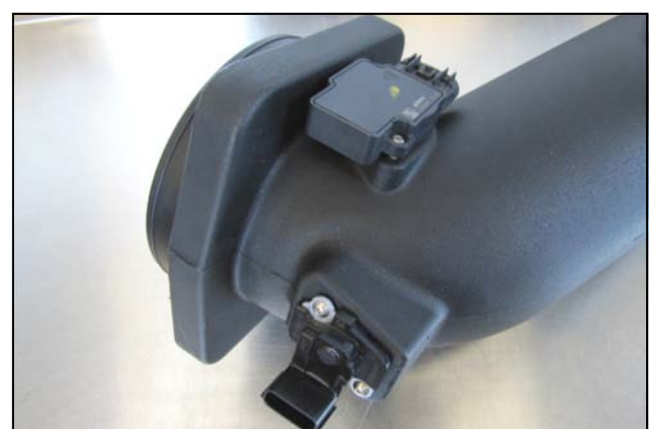
6. Transfer the Mass Air Flow sensors into the Airaid intake Tube and secure them using two 8-32 x 1/2" Button Head Screws. Do Not Use Factory Screws!
