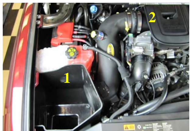
12. Slide the Intake Tube down and into the Cold Air Box, then into the Hump Hose on the turbo inlet.
