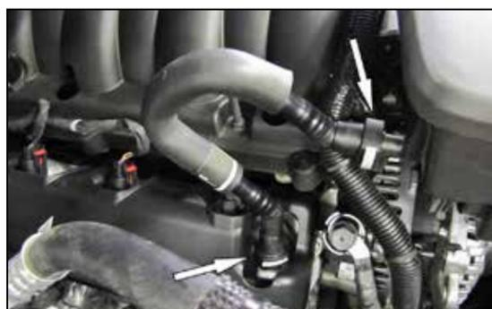
3. Depress the locking tabs and then disconnect the crank case vent line from the intake plenum and valve cover vent port.
