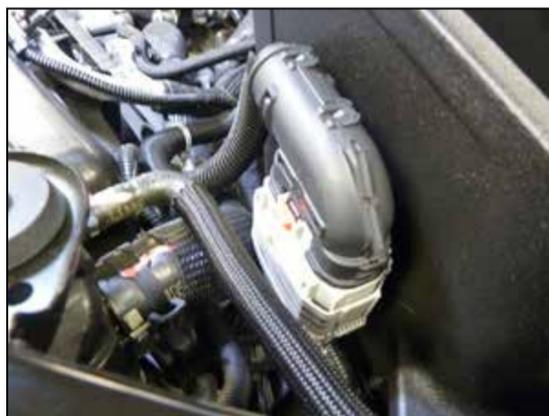
15. Clip the wiring harness onto the bracket installed onto the AIRAID® air filter housing.
