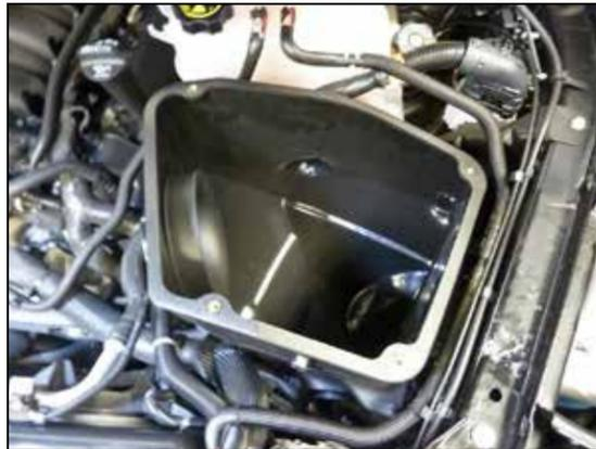
13. Install the AIRAID® air filter housing into the vehicle so the mounting grommets engage into the factory mounting holes. Secure the housing with the factory nut removed in step #9.
