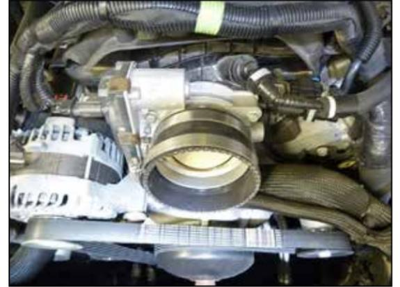
17. Install the appropriate coupler onto the throttle body. The 5.3L engine will use the smaller coupler and the 6.2L engine will use the larger coupler. Secure with the provided hose clamps.
