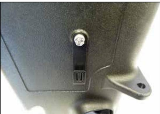
11. Install the provided wiring harness bracket onto the AIRAID® air filter housing and secure with the provided hardware.
