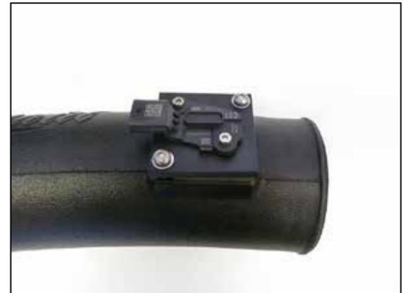
19. Install the mass air sensor assembly into the AIRAID® intake tube in the direction shown and secure with the provided hardware.
