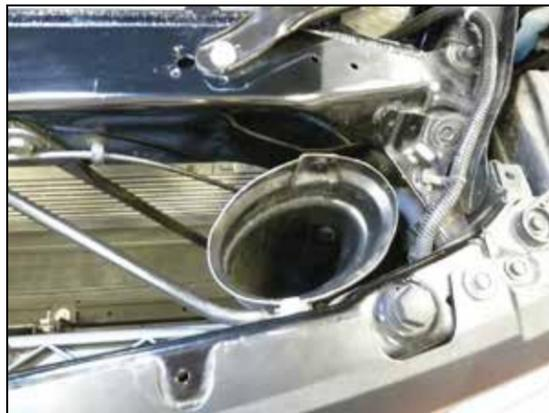
14. Push the factory fresh air intake duct into the AIRAID® air filter housing and then reinstall the plastic clip to secure it into position.
