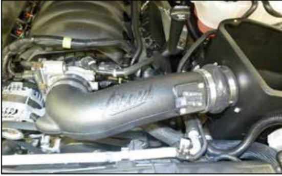
22. Install the AIRAID® intake tube into the coupler at the air filter housing and then into the coupler on the throttle body, adjust the tube for best fit and then secure with the provided hose clamps.
