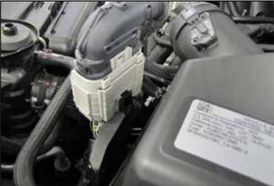
8. Using a small 90° pick or similar tool, release the locking tap that secures the wiring harness bulk connector to the air filter housing and then unhook the connector from the housing. Unhook the wiring harness from the two locations held with tie wraps.
