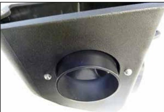
10. Install the provided radius filter adapter into the AIRAID® air filter housing and secure with the provided hardware.
