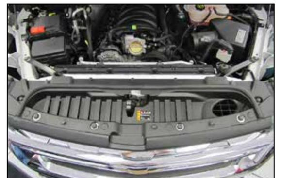
6. Release the ten plastic locking pins holding the upper radiator valence and then remove the valence from the vehicle.
