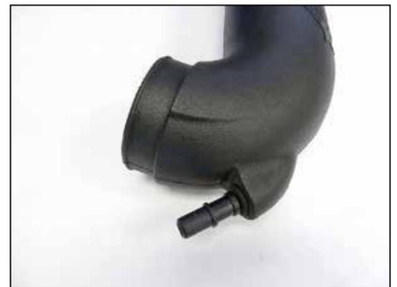
20. Install the grommet and quick disconnect vent fitting into the AIRAID® intake tube as shown.
