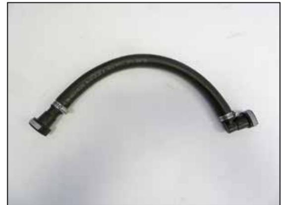
21. Assemble the crank case vent assembly using the provided hose, straight quick disconnect fittings and hose clamps as shown.
