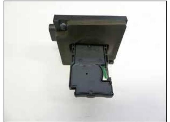
18. Install the provided gasket onto the provided mass air sensor adapter. Remove the mass air sensor from the factory air filter housing and then install it into the adapter and secure with the provide hardware.
