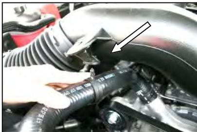
1. **Disconnect the negative battery cable!** Lift up on the front of the and beauty cover and remove it from the vehicle. Push down on the radiator hose, and separate the tube from the plastic clamp.
