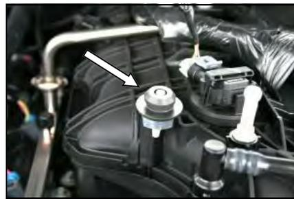
8. Install the grommet from step #7 on the "ball stud", with the small diameter facing up as shown.
