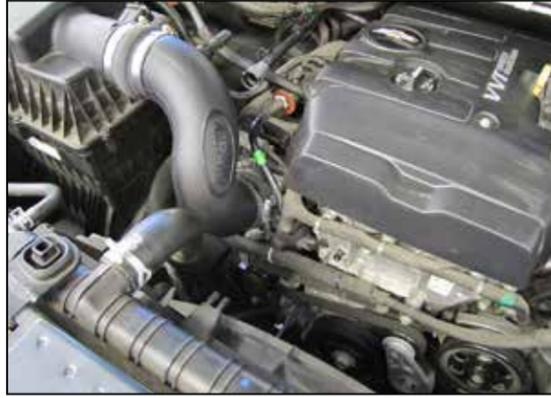
9. Install the intake tube into the coupler at the throttle body, align with the coupler on the air filter housing. Adjust the tube for best fit and secure with the provided hose clamps. Reconnect the crank case vent line.
