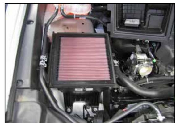
5. Install the AIRAID® air filter and then reinstall the upper housing and secure with the factory screws.
