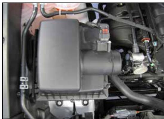
4. Loosen the four bolts that secure the air filter housing lid to the lower housing, set the lid aside and remove and factory air filter.
