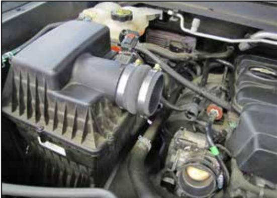
8. Install the provided coupler (08171) onto the air filter housing and secure with the provided hose clamp.
