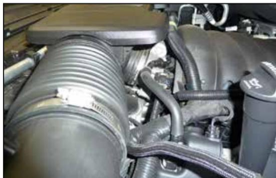
3. Loosen the two hose clamps that secure the intake plenum to the throttle body and then remove the intake plenum from the vehicle.
