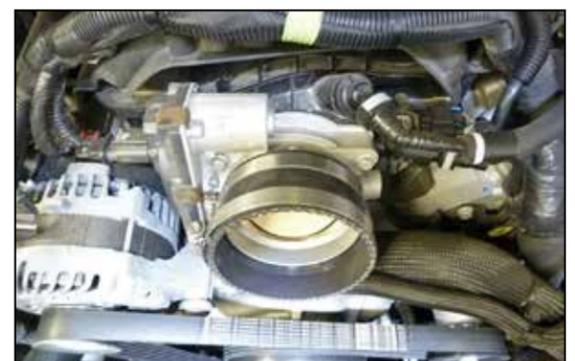
6. Install the provided coupler onto the throttle body. 5.3L engines will use the smaller coupler and 6.2L engines will use the larger coupler.
