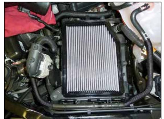
5. Remove the factory air filter and replace with the AIRAID® air filter provided. Reinstall the air filter housing lid and secure with the factory screws.
