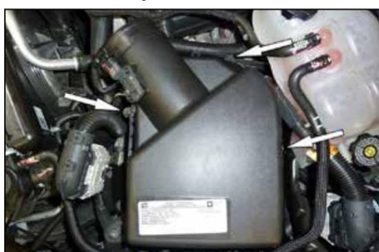
4. Loosen the three screws that secure the air filter housing lid and then lift up the housing and set aside.
