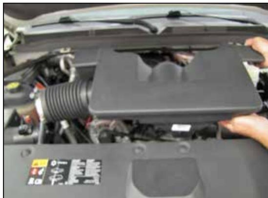
5. Remove the intake plenum from the vehicle.
