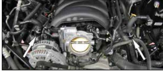
12. Remove the two factory crank case vent tubes from the vehicle.
