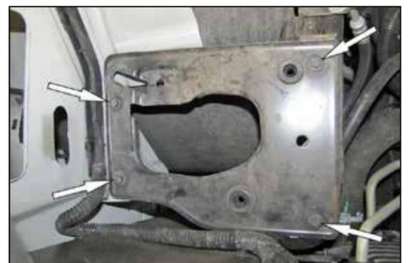
7. Remove the four bolts securing the air box mounting tray and then remove the tray from the vehicle.
