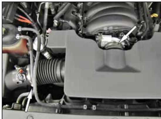
4. Loosen the two hose clamps securing the intake plenum to the factory air box and to the throttle body.
