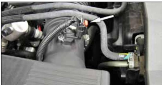
2. Disconnect the mass air sensor electrical connector.
