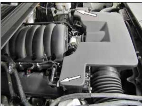
3. Disconnect the two crank case vent tubes from the intake plenum.
