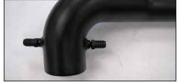
17. Install the two provided crank case vent fittings into the AIRAID intake tube as shown.
