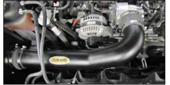
18. Install the AIRAID intake tube into the hose at the filter adapter and then into the hose at the throttle body, adjust the tube for best fit and then secure with the provided hose clamps.
