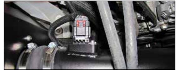
20. Reconnect the mass air sensor electrical connection.
