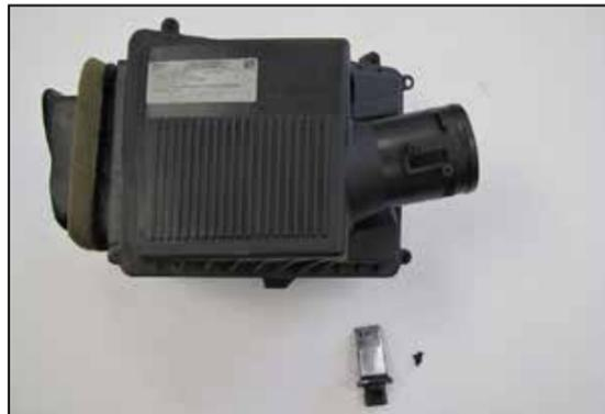
15. Remove the mass air sensor from the factory air box.
