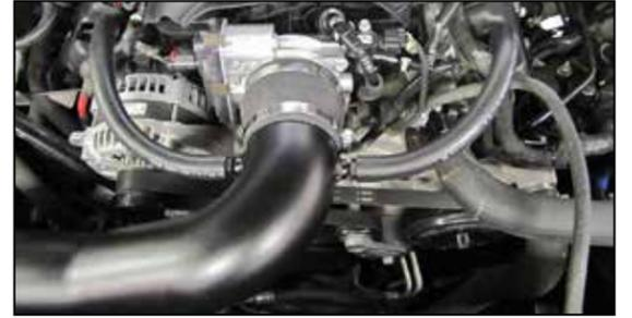
19. Connect the provided crank case vent hoses to the ports on the valve covers and then connect the open ends to the fittings installed into the AIRAID intake tube.
