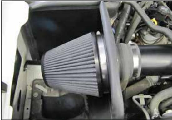
24. Install the AIRAID® air filter onto the filter adaptor and secure with the provided hose clamp.
