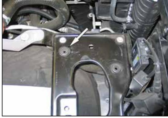
12. Remove the air box mounting grommet shown from the air box mounting plate.
