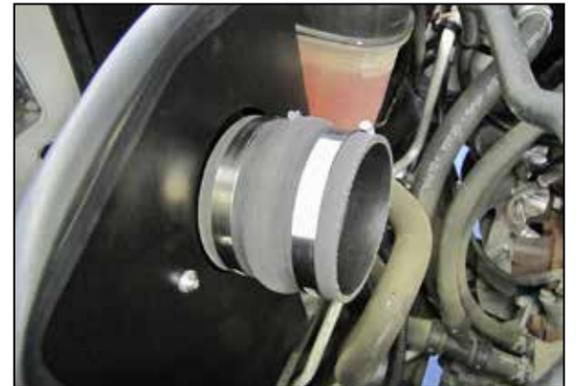
19. Install the provided hump coupler hose onto the filter adapter and secure with the provided hose clamp.
