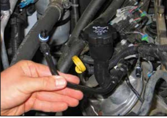
7. Rotate the crankcase vent line on the valve cover port, and then release the locking tab and remove the crankcase vent line from the valve cover.
