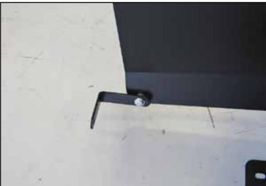
10. Install heat shield mounting bracket onto the heat shield as shown using the provided hardware.
