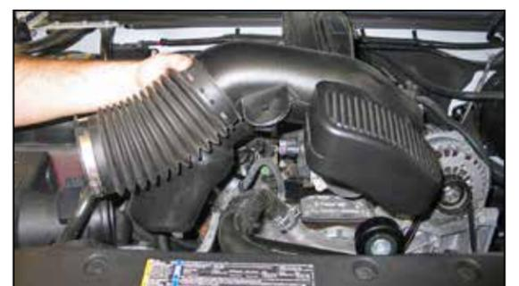
6. Loosen the hose clamp which secures the stock intake tube, then remove the intake tube from the vehicle.
