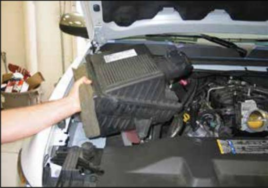
8. Pull firmly upward to release the air filter housing from the mounting tray grommets. Then remove the assembly as shown.
