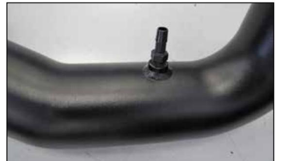
21. Install the provided 1/4" NPT fitting into the AIRAID® intake tube as shown.
