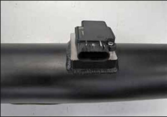
9. Remove the two screws securing the mass air sensor to the air box and then remove the mass air sensor from the air box as shown. Install the mass air sensor into the AIRAID® intake tube and secure with the provided hardware.
