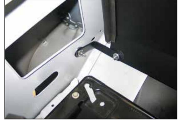
17. Secure the mounting bracket to the inner fender with the hardware provided.
