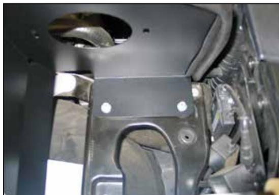
16. Reinstall the heat shield assembly onto the air box mounting plate and secure the two 5/16" bolts provided.
