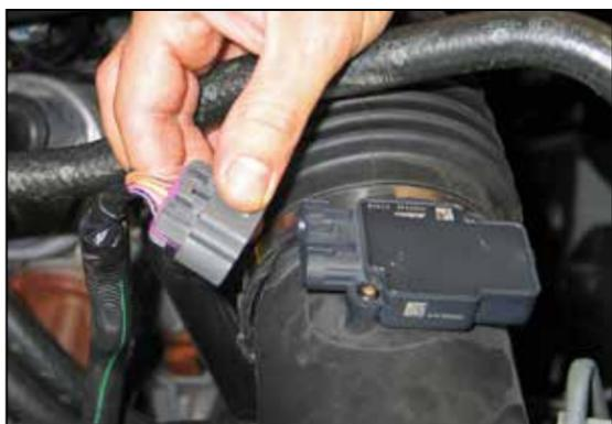
2. Disconnect the mass air electrical connection.
