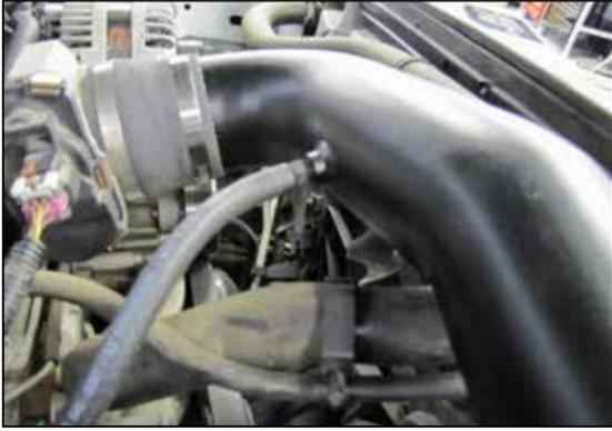
23. Install the provided crankcase vent hose onto the valve cover vent port and then connect the remaining open end to the 1/4" NPT fitting in the AIRAID® intake tube.
