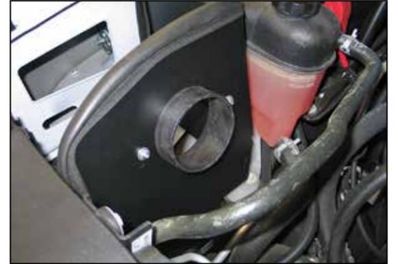
18. Install the filter adapter onto the heat shield and secure with the provided hardware.
