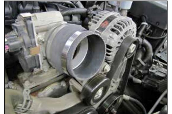
20. Install step coupler hose onto the throttle body and secure with the provided hose clamp.
