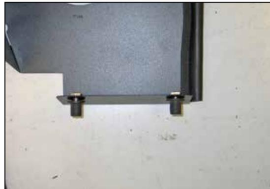
15. Remove the heat shield assembly and drill a 5/8" hole at the marked location. Install the remaining 5/16" inserted nut into the heat shield as shown.
