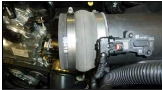
11. Install the AIRAID air filter and then reinstall the upper housing and secure with the factory screws. Install the provided hump coupler onto the air filter housing and secure with the provided hose clamp.
