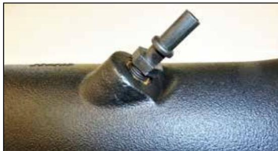
13. Install the provided quick connect fitting into the K&N intake tube.
