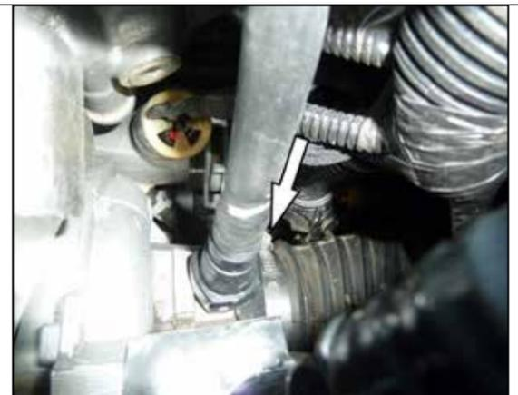
5. Loosen the hose clamp that secures intake tube to the turbo inlet.
