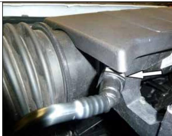
3. Depress the locking tab and then disconnect the CCV pipe from the plenum.
