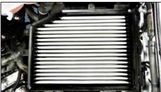
10. Remove the upper air filter housing and remove the factory air filter.
