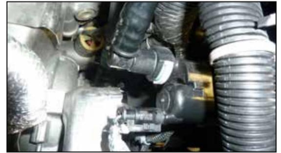
17. Connect the CCV tube to the solenoid and connect the electrical connection.
