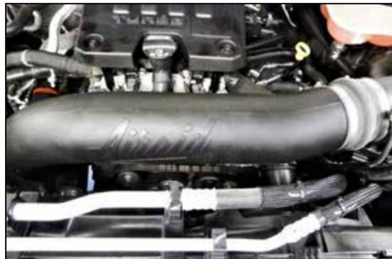
15. Install the intake tube assembly into the coupler at the air filter housing and then into the coupler at the turbo inlet, adjust the tube for best fit and then secure with the provided hose clamps.
