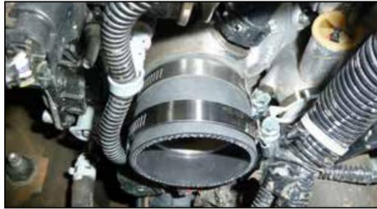
12. Install the provided straight coupler onto the turbo inlet and secure with the provided hose clamp.
