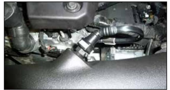
16. Connect the CCV tube to the quick connect fitting installed into the K&N intake tube.
