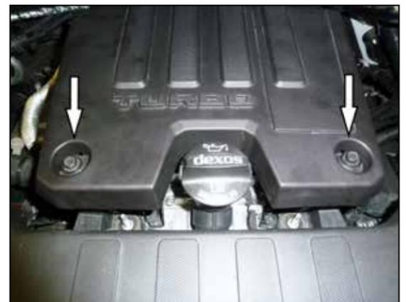
6. Remove the two bolts that secure the engine cover to the engine and then remove the cover from the vehicle. These bolts will be reused in a later step.
