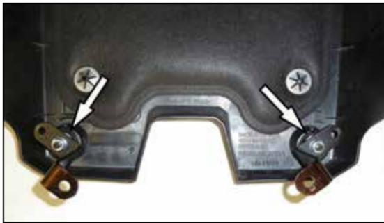
8. Using the factory bolts and the nuts provided, secure the two provided "Z" brackets to the engine cover as shown.
