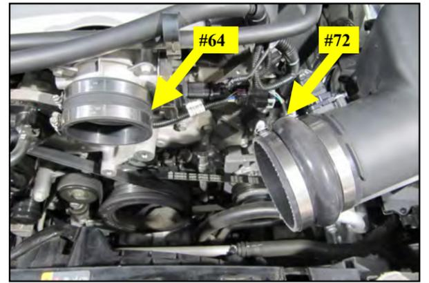
12. Slide the Coupler and the 64 Clamps onto the throttle body and the Hump Hose with the 72 Clamps onto the airbox outlet.
