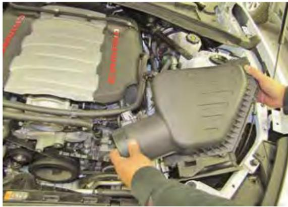
11. Detach and lift the airbox lid and replace the air filter with the provided AIRAID air filter.
