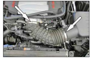
3. Loosen the two hose clamps that secure the factory intake tube and then remove the intake tube from the vehicle.
