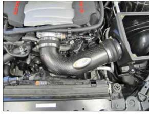
18. Install the coupler houses and hose clamps onto the AIRAID intake tube but do not tighten the clamps. Install the intake tube assembly onto the filter adapter and throttle body. Adjust the assembly for best fit and then secure all the hose clamps.
