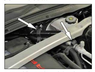
7. Locate and disconnect the sound tube retainers on the strut tower brace and A/C line.
