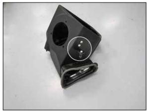
11. Install the provided air filter housing bracket onto the AIRAID air filter housing and then install the provided mounting stud onto the bracket as shown.
