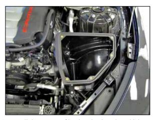
17. Install the AIRAID filter housing into the vehicle so that the mounting posts are engaged into the factory filter housing mounting grommets.
