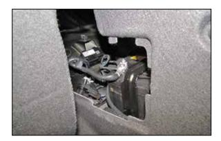
1. Inside the trunk, on the passenger side, locate and remove the access panel for the battery. Disconnect the negative battery cable. NOTE: Vehicle shown is a convertible.
