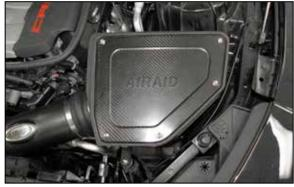
22. Install the air filter housing lid onto the AIRAID air filter housing and secure with the provided hardware.
