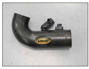
16. Install the PCV chamber into the grommet previously installed into the AIRAID intake tube as shown.
