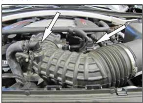
2. Release the spring clamp securing the resonator tube to the 90 deg. Fitting and then disconnect the tube. Depress the locking tab and then disconnect the crank case vent hose.
