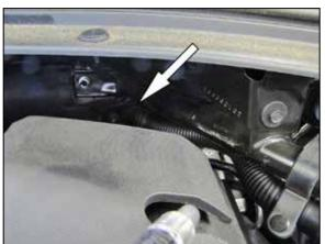
8. At the firewall, Remove the 6mm flange nut that secures the sound tube to the firewall. Turn the tube ½ turn clockwise and the remove the tube from the vehicle.
