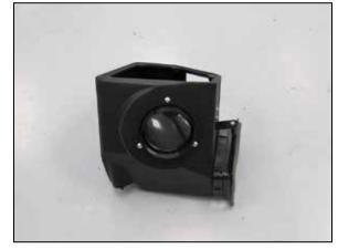
12. Install the radius filter adapter into the AIRAID filter housing and secure with the provided hardware.
