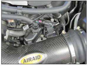
19. Connect the crank case vent hose to the PCV vent chamber and connect the mass air sensor electrical connection.
