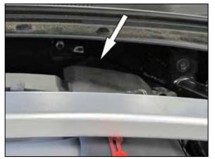
9. Install the provided plug into the sound tube hole.
