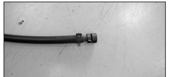
18. Install the provided quick disconnect fitting into one of the provided coolant hoses and secure with the provided spring clamp.
