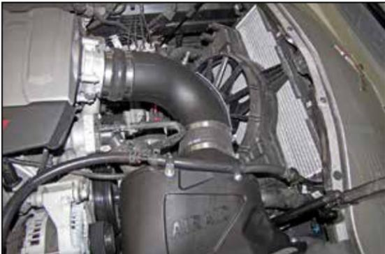
23. Install the AIRAID® intake tube into the straight coupler at the mass air sensor and then into the hump coupler at the throttle body, adjust the tube for best fit and then secure with the provided hose clamps.
