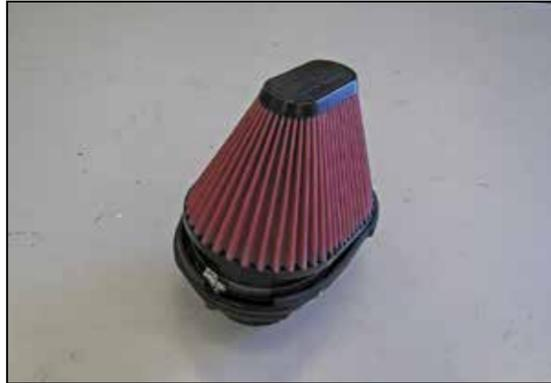
13. Install the AIRAID® air filter onto the AIRAID® mass air sensor assembly and secure with the provided hose clamp.
