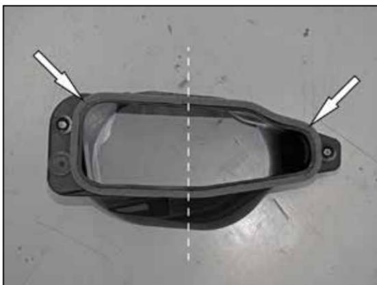
10. Install the foam gaskets onto the AIRAID® air filter housing in the location shown.
