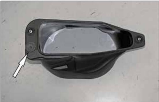
9. Transfer the factory air filter housing mounting grommet to the AIRAID® air filter housing in the location shown.
