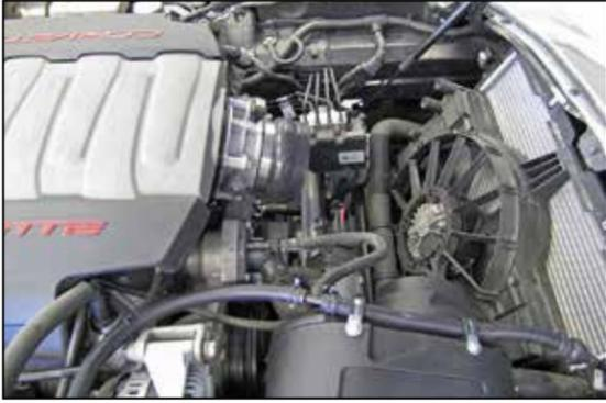
21. Install the provided hump coupler onto the throttle and secure with the provided hose clamp.
