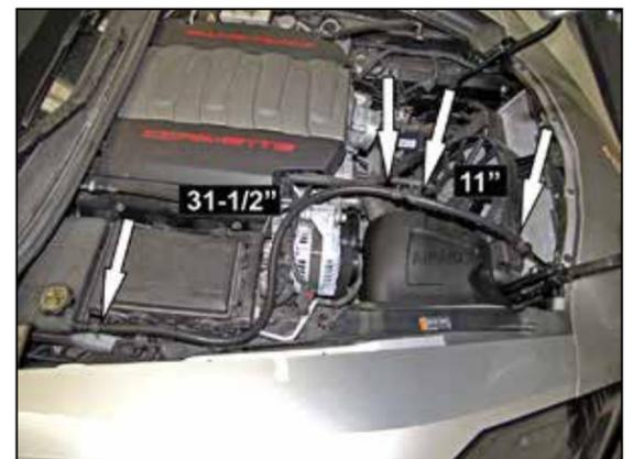
19. Trim the hose with the quick disconnect fitting to 31-1/2" long and trim the remaining hose to 11" long. Install the 31-1/2" long hose from the expansion tank to the tee fitting. Secure the hose with the provided spring clamp, route the hose as shown and secure with the provided tie wraps. Install the 11" hose onto the check valve and tee fitting and secure with the provided spring clamps.
