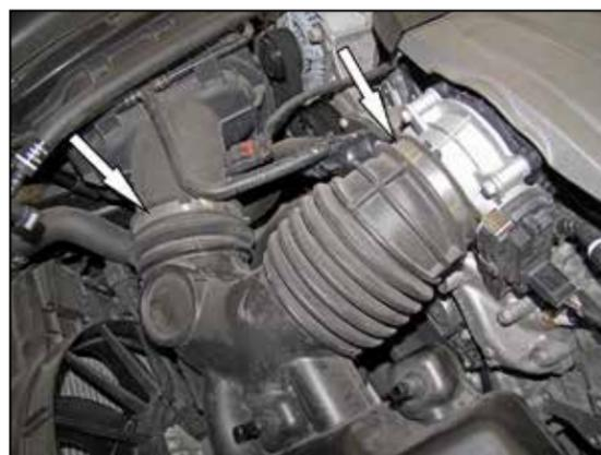
4. Loosen the two hose clamps that secure the factory intake tube to the throttle body and air filter housing and then remove the tube from the vehicle.
