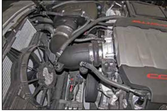
24. Connect the crank case vent hoses onto the fittings installed into the AIRAID® intake tube.
