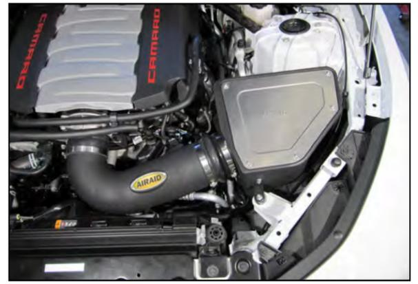
27. Slowly lower the hood to test clearances. Make sure all clamps, hoses, bolts, and screws are tight. Double check the hood clearance. Reconnect the negative battery terminal and re install the access panel.
