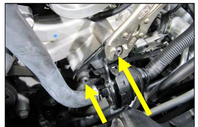
6. Remove the two bolts in the resonator diaphragm bracket using a T-50 Torx bit or with a pair of locking pliers as shown. The resonator, bolts and bracket will not be used with the Airaid.
