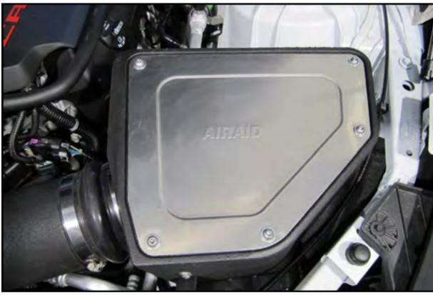
25. Remove the protective film from the other side of the Lid and mount it to the Airbox using 5 sets of 1/4-20 Button Heads and Flat Washers.
